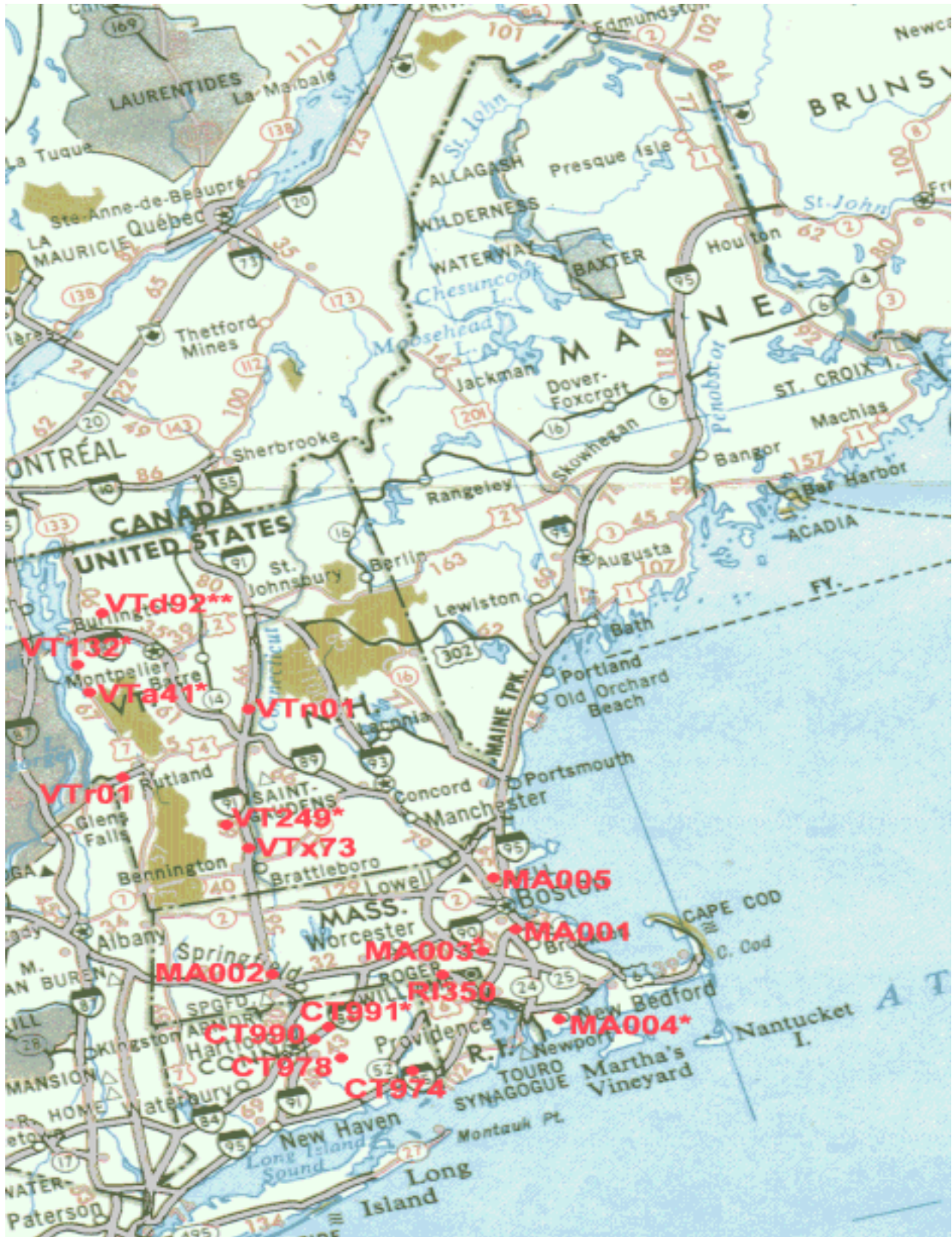
Figure 1.1. The Seventeen Classification/WIM Sites Kept for Analysis. *Classification analysis only; **WIM analysis only; other sites were used in both analyses.
