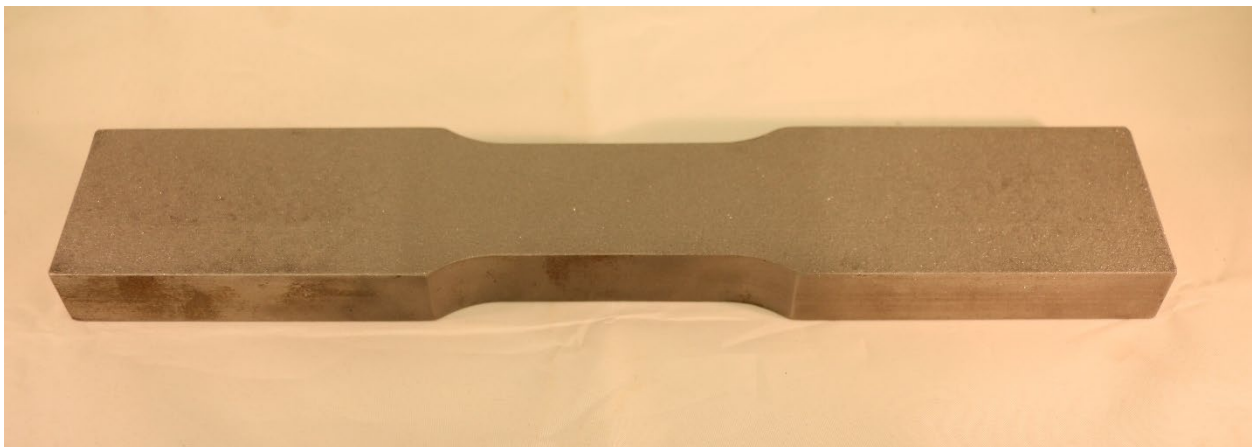
Figure 4. Photo. Typical steel tensile test coupon.
