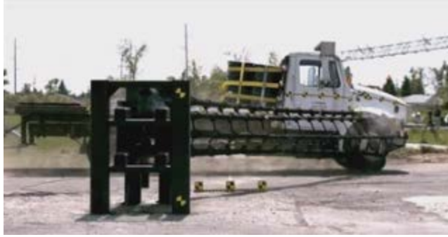
Figure 31. Photo. Active arresting barrier.
