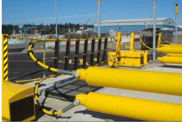
Figure 3. Photo. Active arresting barrier.
