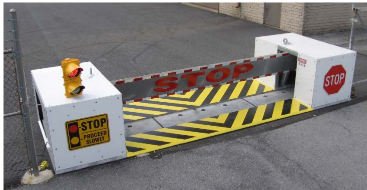
Figure 6. Photo. Example of a portable/movable active VSB.
