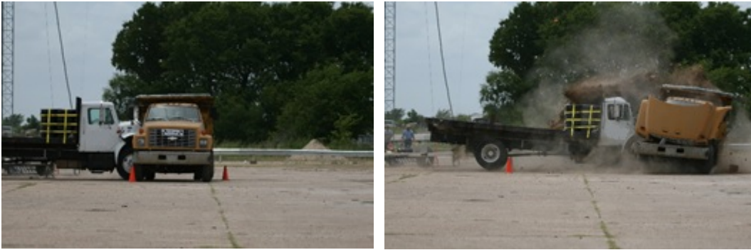
Figure 39. Photos. Single-axle highway vehicle barrier standard test truck performance test.
