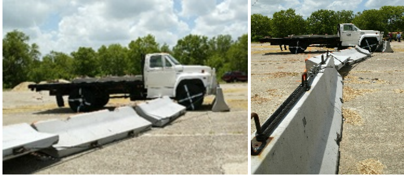
Figure 23. Photos. 2003 USAF and DOS test conducted at 30 mph versus original DOS standard.
