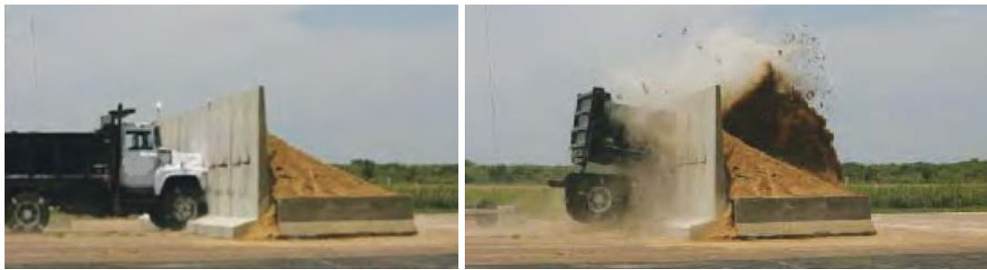
Figure 24. Photos. Heavy goods vehicle performance test.
