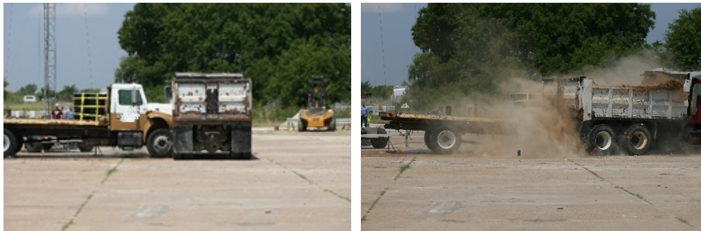
Figure 38. Photos. Dual-axle highway vehicle barrier standard test truck performance test.
