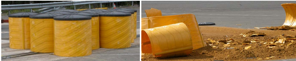
Figure 26. Photos. Sand-filled highway safety barrels—pre- and post-test against medium-duty truck.
