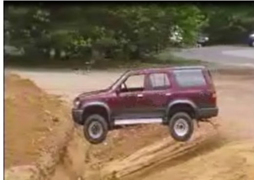
Figure 32. Photo. Anti-vehicular ditch with berm.
