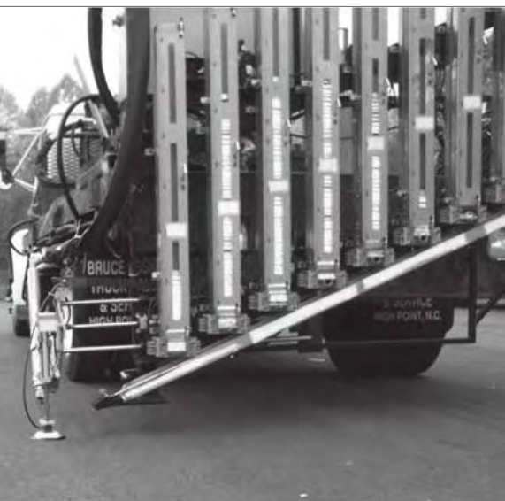
The intelligent asphalt compaction analyzer is mounted on compaction equipment to provide real-time data so problems can be fixed during the paving process.
