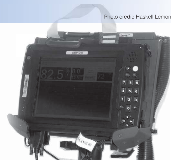
The Intelligent Asphalt Compaction Analyzer measures asphalt pavement density in real time, allowing equipment operators to fix problems before the asphalt hardens.
