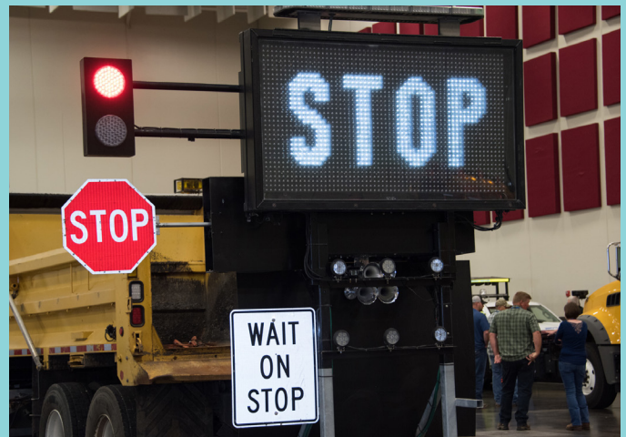
The TMA Flagger is operated from a truck cab, eliminating the need for a human flagger on the road.
