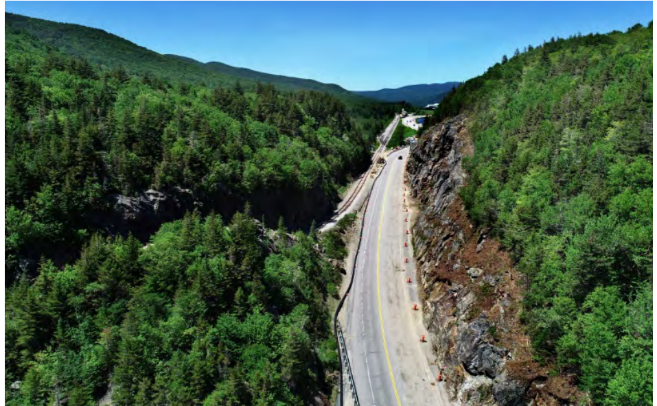
The New Hampshire Department of Transportation combined drone photos with photogrammetry from its A-GaME toolbox to characterize rock structure conditions on Route 302.
