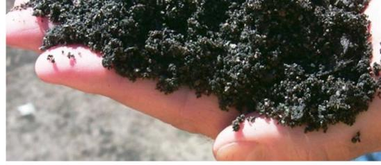
This handful of processed shingles, or RAS, is ready for inclusion in an asphalt mixture. *Source: Astec Industries.*
