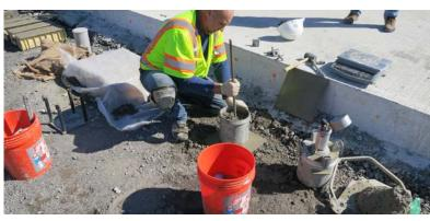
A technician from the Mobile Concrete Trailer is preparing a fresh concrete sample for air void testing at a project site. *Source: APTech.*
