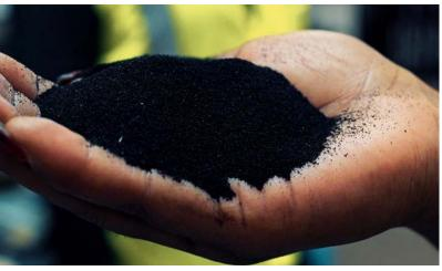
A handful of rubber powder produced from ground up tires. Source: Lehigh Technologies, Inc.
