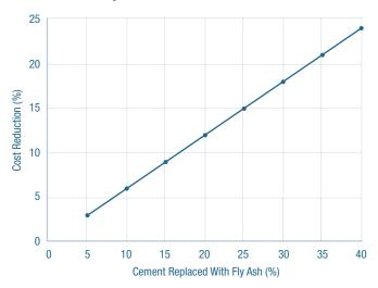
Note: Savings are per ton of cementitious materials used and assume 1:1 replacement. Unit cost of cement is assumed to be \$100 per ton, while fly ash is \$40 per ton.
