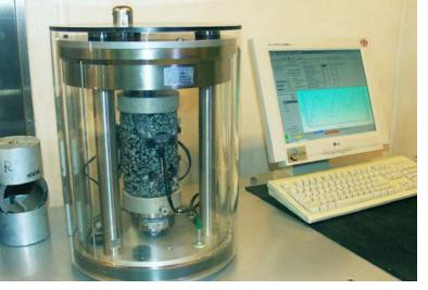
Using advanced testing equipment inside the Mobile Asphalt Trailer, FHWA technicians can provide valuable feedback to agencies on the performance of their mixtures containing increased percentages of recycled materials. *Source: Matthew Corrigan, FHWA.*
