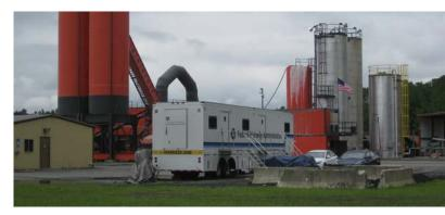
FHWA's Mobile Asphalt Testing Trailer, shown here at a plant in Lake City, FL, recently visited projects in Florida and Arizona to evaluate the performance of GTR. The mobile testing trailer also supported the American Association of State Highway and Transportation Officials and ASTM International in revising the standards for evaluating binders incorporating GTR.
