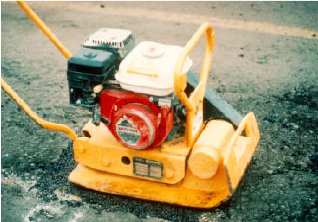
Figure 5. Semi-permanent procedure—compaction using vibratory-plate compactor.
