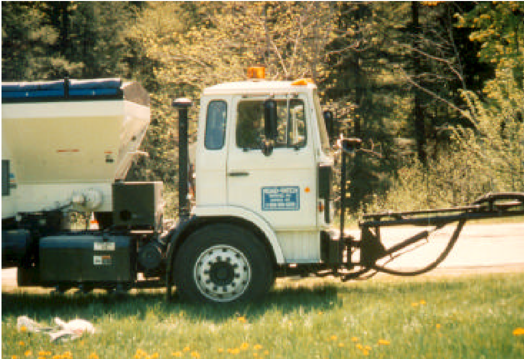
Figure 8. Spray-injection device—self-contained unit.
