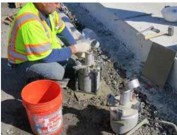
e. Air test (Super-Air Meter [left] and Standard Volumetric Air Meter [right]).
