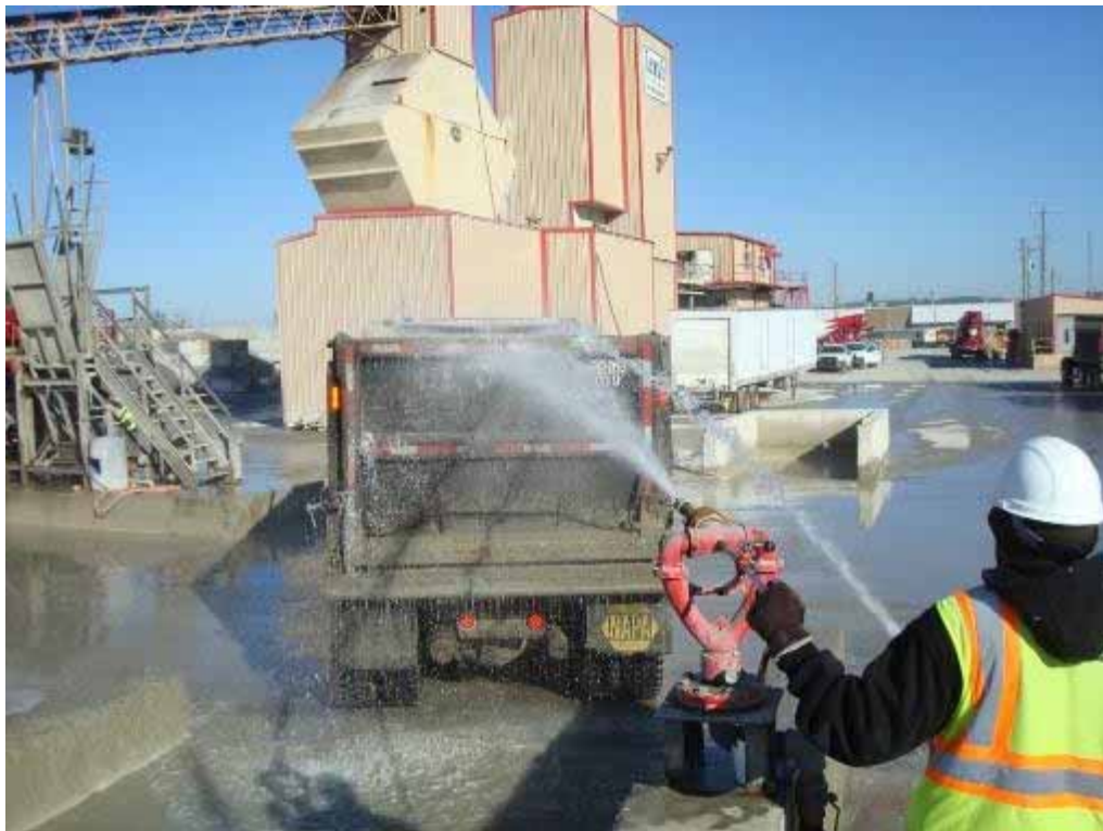
Photo E-10. Truck wash station at IMI ready-mix facility.
