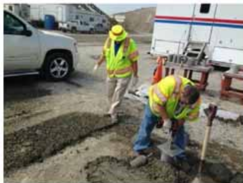
Figure 29: AVA sample being taken from a cylinder
