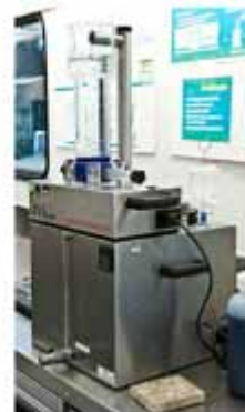
Figure 30: The Air Void Analyzer (AVA)
