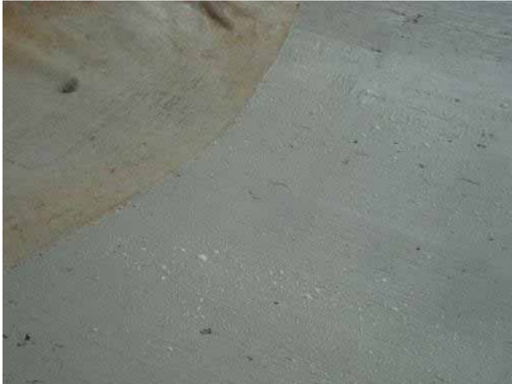
Photo E-34. Free water and bubbles on surface of bottom lift due to excessive water application to burlap drag.
