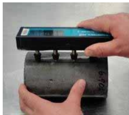
Figure 37: Surface Resistivity Meter in Operation
