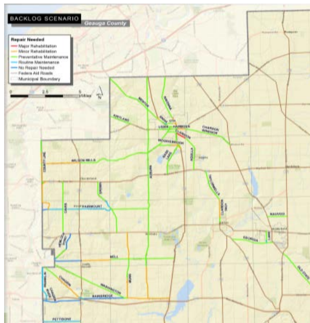
Figure 7. Geauga County's conditions.
