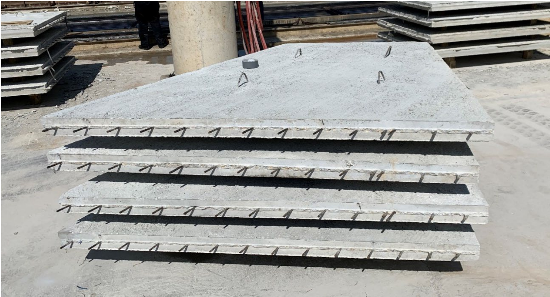
Figure 29. Photo. Skewed end panel with strands parallel with skewed end.
