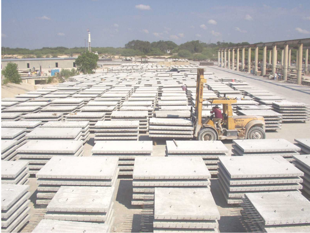
Figure 36. Photo. Aging of panels in storage yard.
