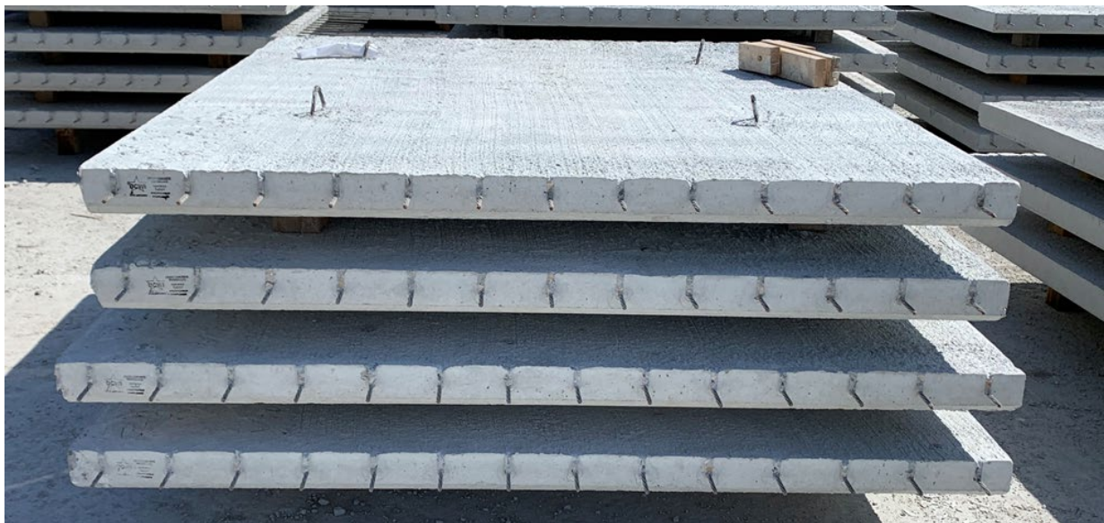
Figure 9. Photo. Typical strand extension from PDDP panels.
