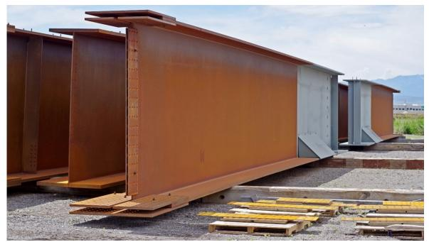
Figure 19: Photo. Fabricated steel plate girders for the I-80 bridges in the fabrication yard.
