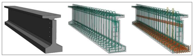
Figure 23: Illustration. Three levels of development for a prestressed beam.
