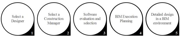
Figure 16: Flowchart. Steps taken to initiate the BIM process.
