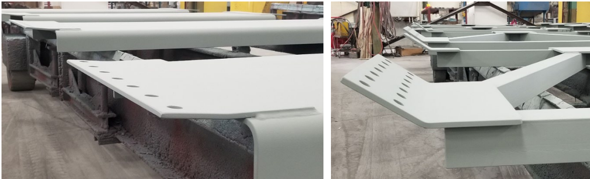
Figure 129. Photos. Bent gusset plates.
