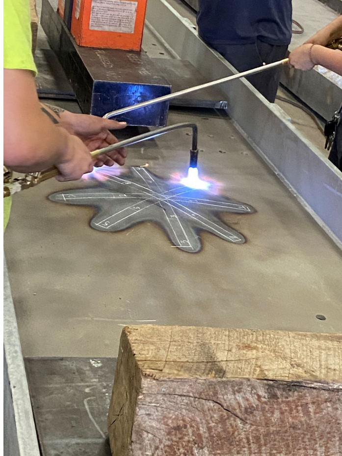
Figure 52. Photo. Web distortion repair with line heats.
