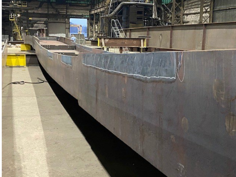
Figure 51. Photo. Horizontal heat curving with strip heats.
