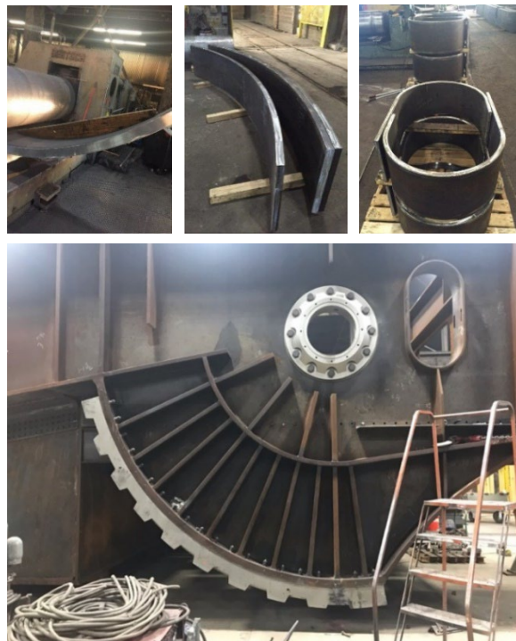
Figure 123. Photos. Cold bent bascule bridge components.
