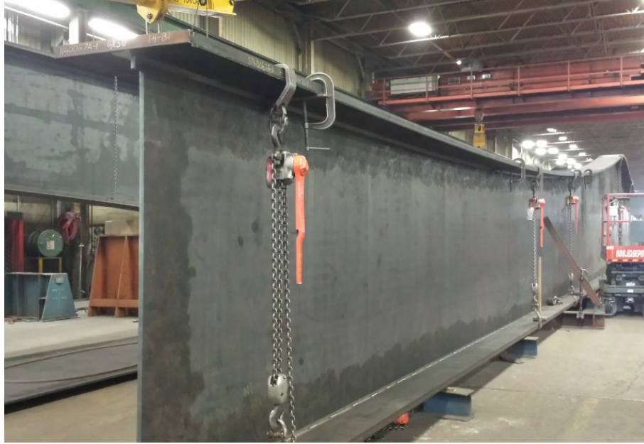
Figure 121. Photo. Haunched girder in fabrication (upside down).
