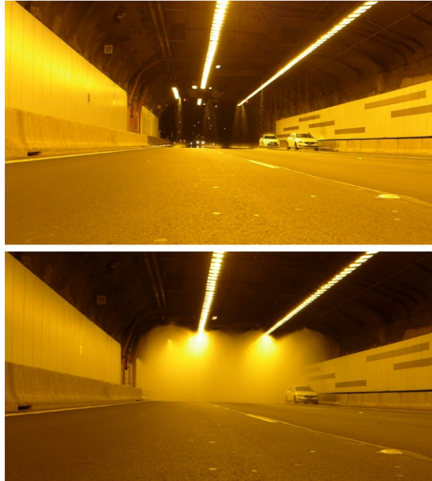
Figure 4-11: Effect of FFFS on visibility [15].
