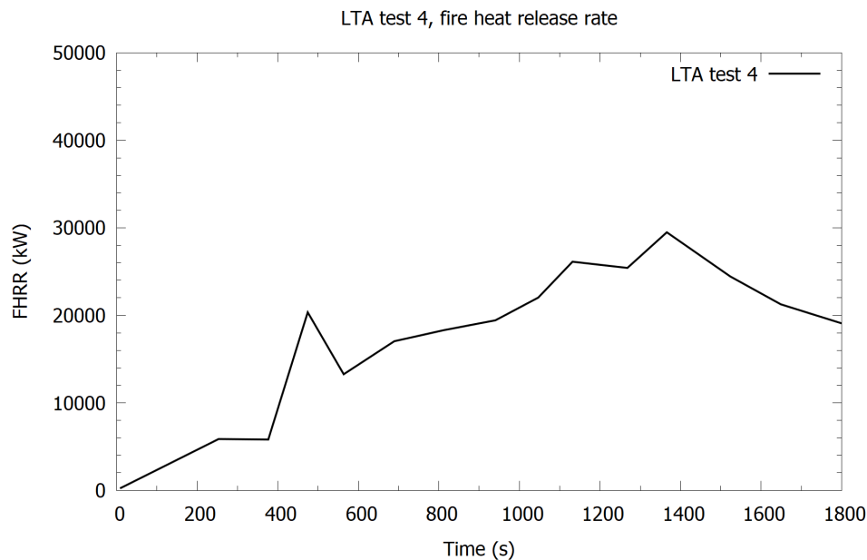
Figure 4-8: Fire heat release rate profile with FFFS operating (LTA test 4) [8].
