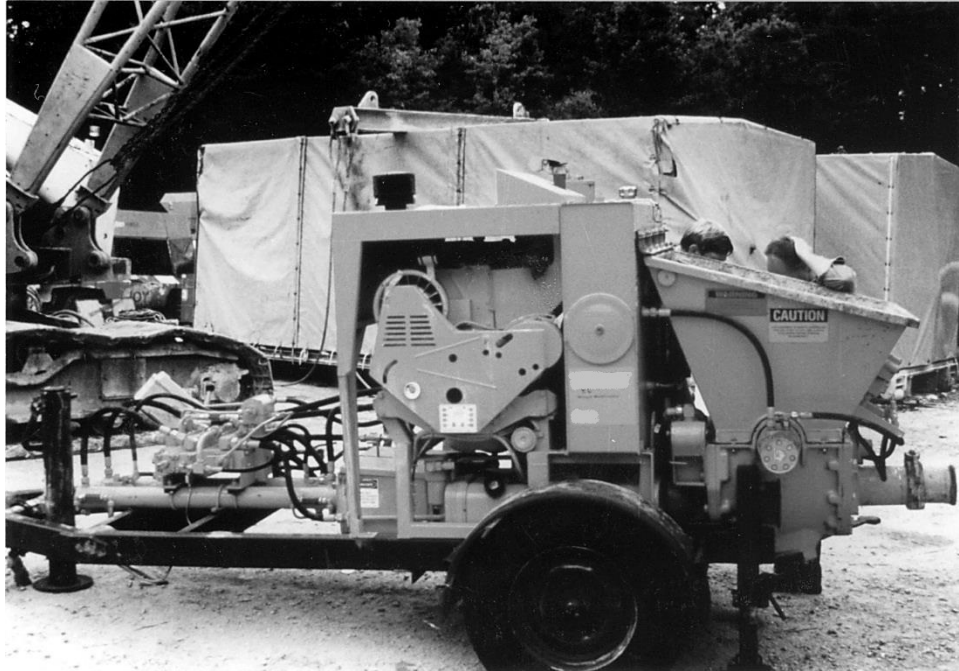
Figure 8-41. Compaction grout pump.
