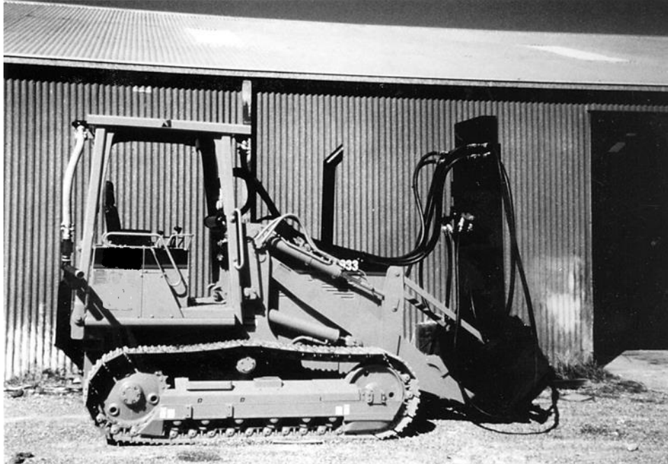
Figure 8-47. Hydraulic crawler rig for lime injection.
