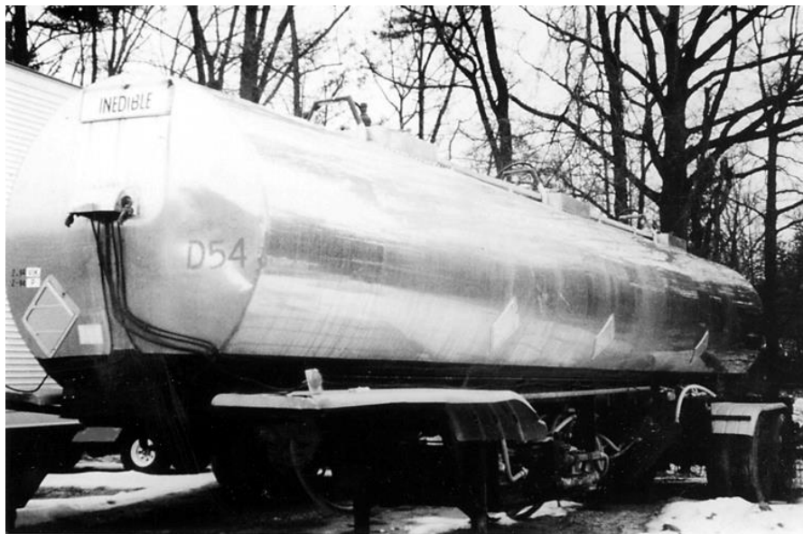
Figure 8-42. Compartmentalized tanker for raw chemical grout components.
