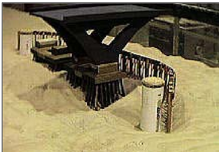
Figure 10.12. Photograph of the post-scour condition of a small-scale physical model test of a Woodrow Wilson Bridge pier.
