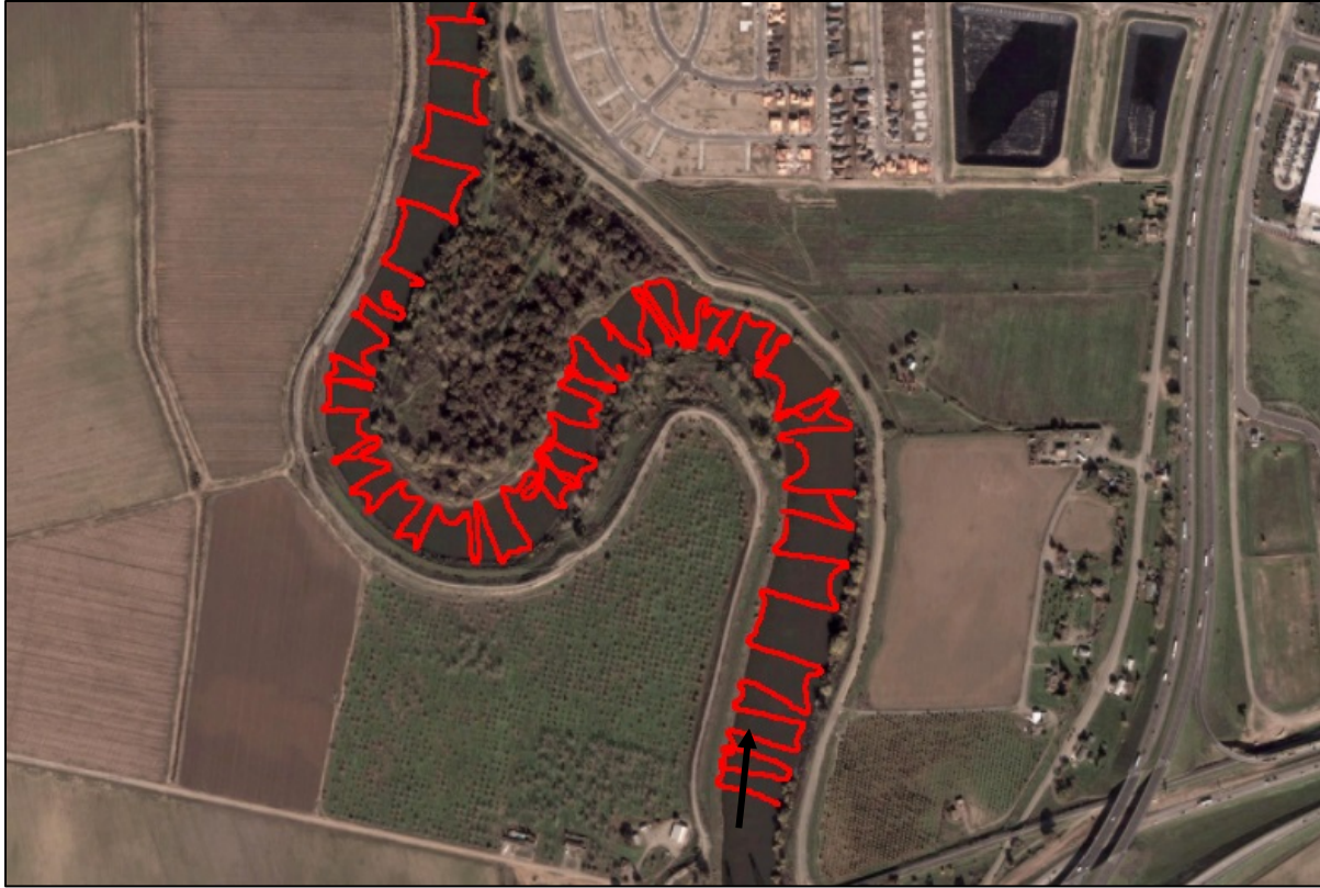
Figure 4.18. Single-beam bathymetric data points, unprocessed.
