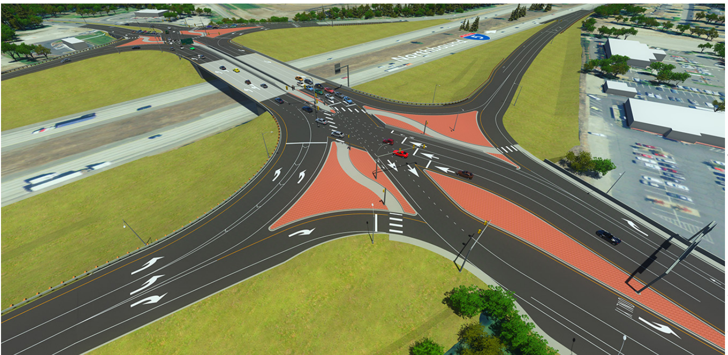
Still-image renderings and other products generated from a 3D model help people visualize Washington State’s first diverging diamond interchange.
