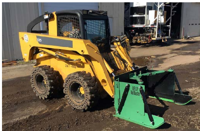
The RutBuster attachment helps fill ruts in asphaltic roadway wheelpaths quickly and efficiently.
