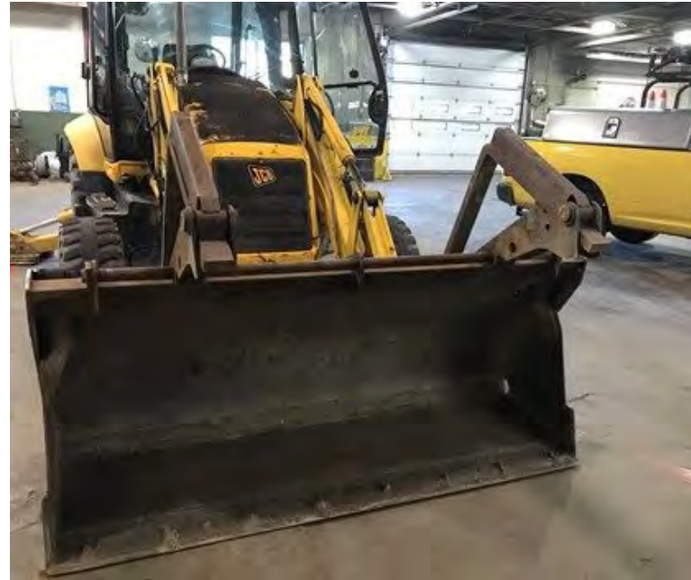
Forks folded over attached to digging bucket of backhoe. Source: PennDOT
