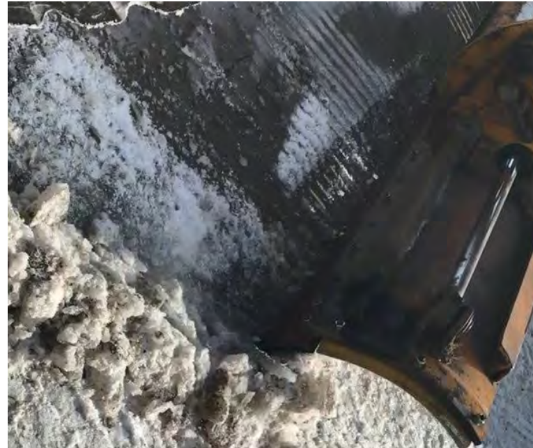
Ice blade uses tines to break up ice for removal. Source: PennDOT
