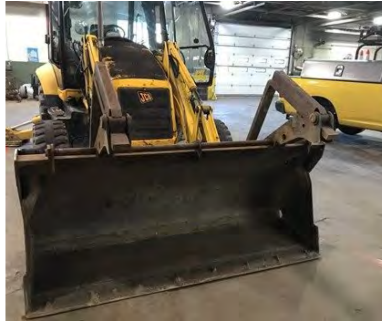
Forks folded over attached to digging bucket of backhoe. Source: PennDOT
