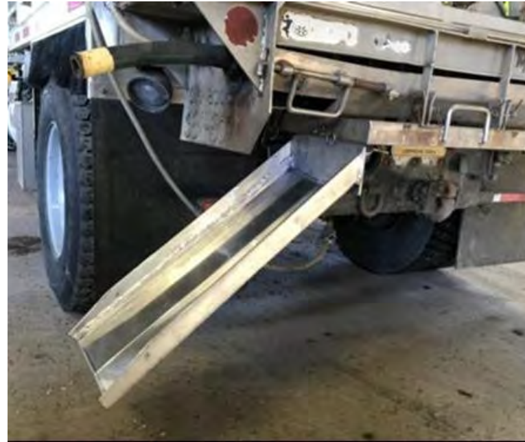
Aluminum device attaches to the spreader. Source: PennDOT
