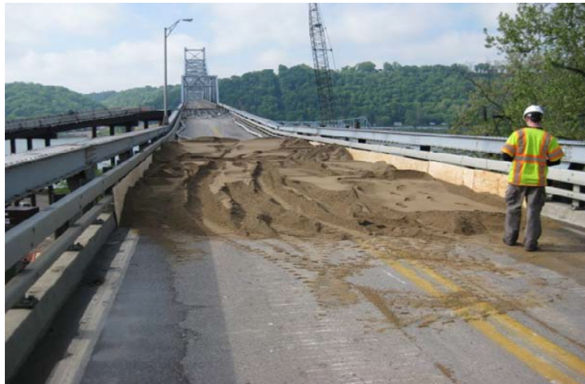
Figure 21. Photo. Sand loading on the Milton–Madison Bridge (FHWA 2013).
