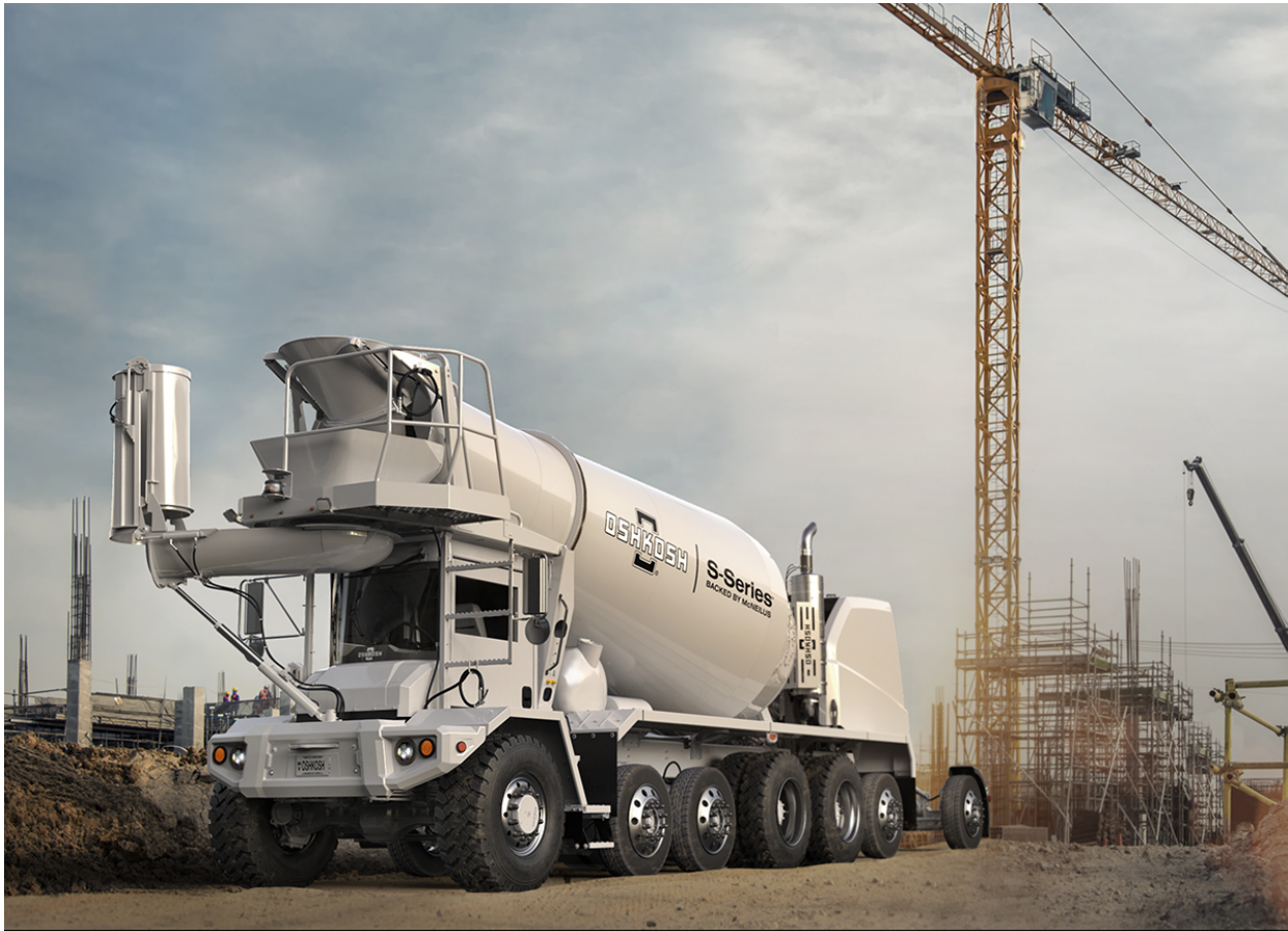
Figure 50. Photograph. Example of a six-axle concrete mixer.
