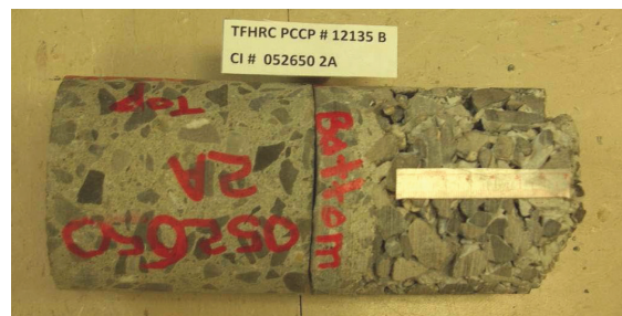
Figure 9. Photograph showing the top and bottom ends of a section of concrete from I-90.
