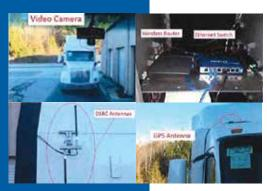
Photo credit: © n.d. Auburn University, College of Engineering. CACC system incorporates video cameras, a dedicated short-range communication system for inter-vehicle data exchange, and GPS.
