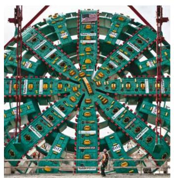
Figure 2. Photo. Tunnel boring machine nicknamed "Bertha" being lowered into position to begin 2-mile-long tunnel project in Seattle, WA, July 2013. ©Washington State Department of Transportation.
