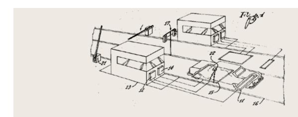
Figure 5. Illustration. Automatic toll charging system, U.S. Patent 3602881. Technology that makes electronic toll collection possible was patented in 1971. Source: United States Patent and Trademark Office, www.uspto.gov.
