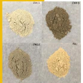
© College of Engineering, Georgia Institute of Technology. Researchers tested several commercially available alternatives to portland cement, including the four pictured here, clockwise from top left: a calcium sulfoaluminate cement (CSA2), a calcium aluminate cement (CAC3). a ternal blend of portland cement, calcium aluminate cement, and calcium sulfate (CAC2), and a chemically activated binder produced with Class C fly ash (AA1).
