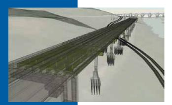
© Civil, Architectural & Environmental Engineering, Drexel University. Researchers at Drexel University are developing a virtual laboratory in which users examine and study the conditions of virtual bridges. Each virtual bridge, like the one pictured above, is the digital twin of a real-life bridge.
