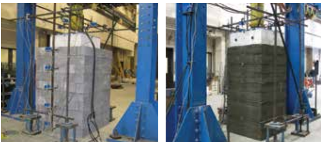
Minipier tests helped quantify SLS for GRS with (left photo) and without (right photo) concrete masonry facing.
