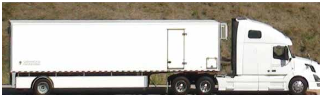
The Traffic Speed Deflectometer is a trailer truck that measures pavement dynamic responses while traveling at traffic speed.
