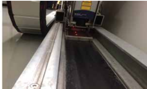
Internal pavement response measure instrumentation of the Traffic Speed Deflectometer.
