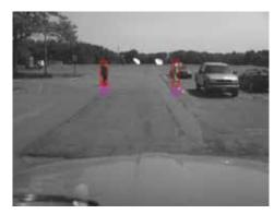
Visual output of the pedestrian-detection system as it recognizes crossing pedestrians. Source: FHWA.
