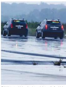
FHWA test vehicles simulate a "platoon" of vehicles using cooperative adaptive cruise control. Source: FHWA.
