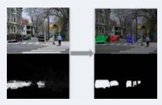
A typical challenging situation for overlapping objects (left vehicles) and occluded objects (right vehicle) in an urban environment. © Carnegie Mellon University.
