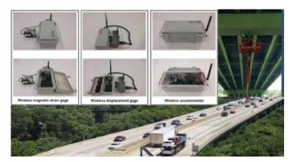
The sensors pictured in the inset image—wireless magnetic stain gauge (left), wireless displacement gauge (middle), and wireless accelerometer (right)—were tested on this 11-span viaduct carrying Interstate 76 west of Philadelphia, PA. © Drexel University.
