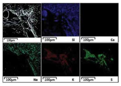
Backscattered electron images of a potassium sulfate crystal formed inside of a silica gel in the interfacial transition zone. The 100  $\mu m$  shown in the image is equivalent to 0.0039 inch. Source: FHWA.
