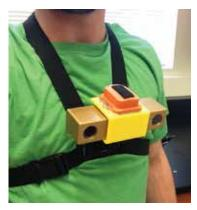
A chest-mounted stereo camera and inertial measurement unit form part of Auburn University's pedestrian navigation system.
