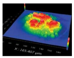
A three-dimensional image acquired using vertical scanning interferometry that shows a cluster of fly ash particles. © Henry Samueli School of Engineering and Applied Science, University of California, Los Angeles.
