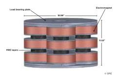
Bearings composed of MRE material sandwiched between electromagnet arrays adjust stiffness and dampening properties in response to strain. © 2016 Proc. SPIE.
