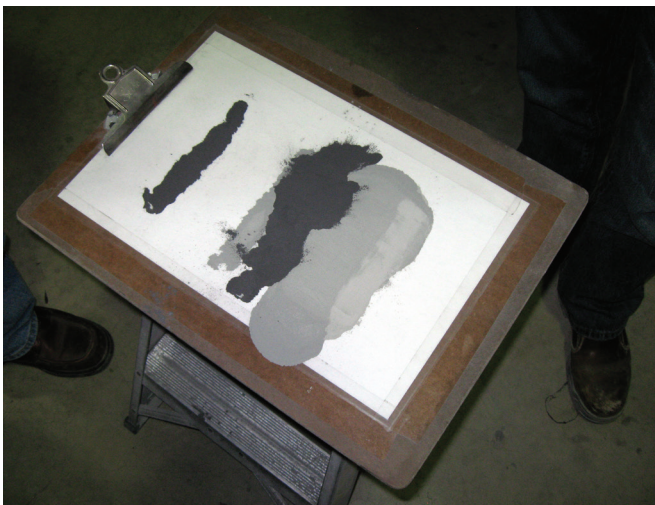
Fly ash with different carbon content levels. Source: FHWA.
