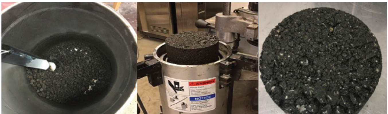
Researchers created a rotary reactor to simulate the production of the hot-mix bio-based binder through mixing aggregates with bioasphalt. © 2017 Department of Civil and Environmental Engineering, Washington State University.
