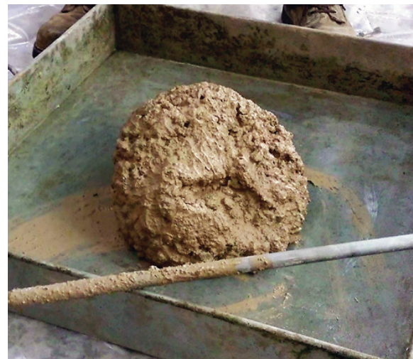
Concrete slump made of an alternative cementitious material (calcium sulfoaluminate). © College of Engineering, Georgia Institute of Technology.
