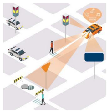
Computer vision can annotate secondary behaviors inside the vehicle, extravehicular context, and interactions between the driver and the environment.  $\ensuremath{\mathbb{C}}$  Virginia Tech Transportation Institute.
