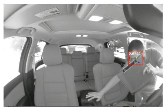
Neural networks can detect faces even under challenging circumstances, such as acute angles and occlusion. © REACTOR Lab.
