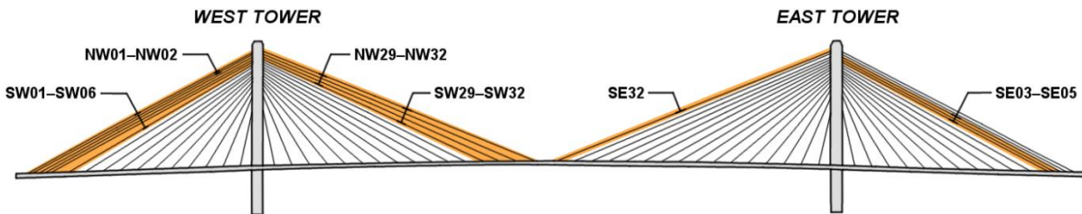
Figure 22. Illustration. Arrangement of cables tested during phase 1.
