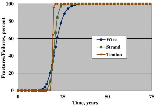
Figure 44. Graph. Percentage of wire and strand fractures and tendon failures as a function of time for the case of sound grout with 0.80 wt% chloride and  $\sigma(CRE)$  on corrosion rate equal to 0.15  $\mu(CRE)$ .
