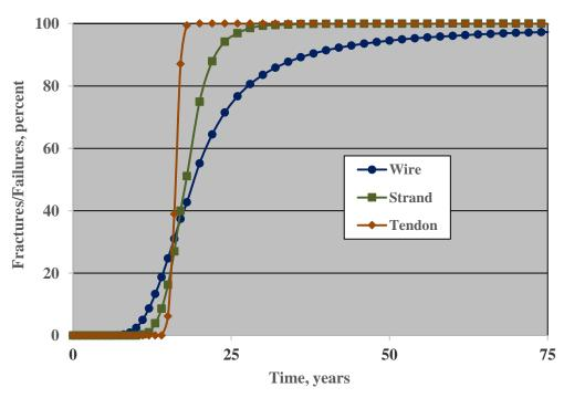
Figure 42. Graph. Percentage of wire and strand fractures and tendon failures as a function of time based on pit depth determinations for phase 1 Specimen Number  $2.0\%-F-S.^{(1)}$
