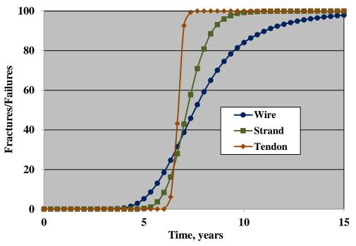
Figure 74. Graph. Plot of the percentage of wire and strand fractures and tendon failures as a function of time based on a mean wire corrosion rate of 10.0 mpy and standard deviation 0.3 of the mean.
