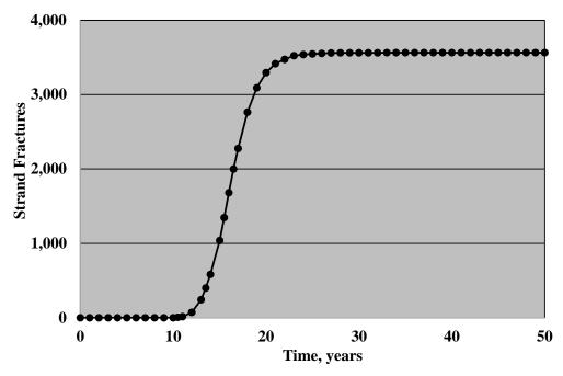
Figure 53. Graph. Plot of the number of strand fractures as a function of time for Specimen Number 1.0%–V–S (grout with 1.0 wt% chloride and an air void).
