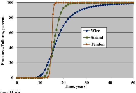
Figure 55. Graph. Plot of the percentage of wire and strand fractures and tendon failures as a function of time based on phase 1 corrosion data for Specimen Number 1.0%-V-S (grout with 1.0 wt% chloride and an air void).(1)
