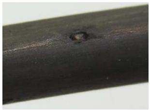
Figure 19. Photo. Example of initial localized corrosion on a wire from a fully grouted single-strand specimen of the phase 1 study (figure 239) for which grout chloride concentration was 0.80 wt% (pit depth is 4.7 mils).<sup>(1)</sup>
