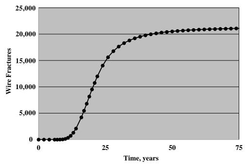
Figure 38. Graph. Number of wire fractures as a function of time for the case of sound grout with 0.80 wt% chloride based on pit depth determinations for phase 1 Specimen Number 0.8%-F-S.<sup>(1)</sup>
