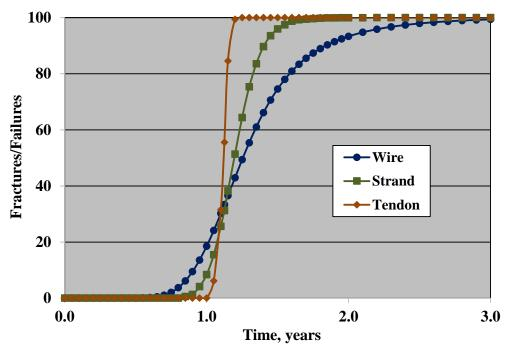
Figure 80. Graph. Plot of the percentage of wire and strand fractures and tendon failures as a function of time based on a mean wire corrosion rate of 60.0 mpy and standard deviation 0.3 of the mean.
