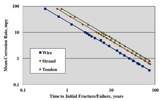
Figure 120. Graph. Plot of  $T_f$  for wires, strands, and tendons as a function of corrosion rate for  $\sigma(CRE)/\mu(CRE)=0.30$ .
