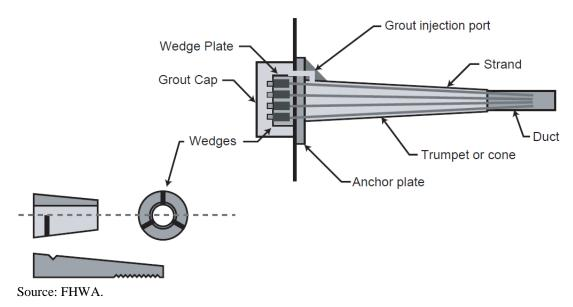
Figure 1. Illustration. Schematic drawing of a PT tendon with various components identified.
