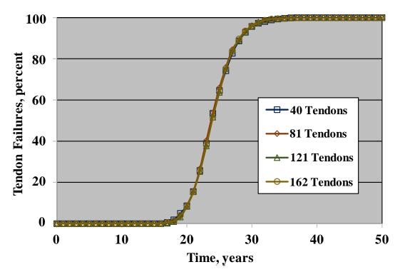
Figure 97. Graph. Plot of the percentage of tendon failures as a function of time for systems with 40, 81, 121, and 162 tendons.
