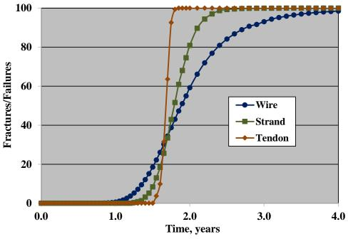
Figure 78. Graph. Plot of the percentage of wire and strand fractures and tendon failures as a function of time based on a mean wire corrosion rate of 40.0 mpy and standard deviation 0.3 of the mean.
