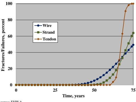
Figure 68. Graph. Plot of the percentage of wire and strand fractures and tendon failures as a function of time based on a mean wire corrosion rate of 1.0 mpy and standard deviation 0.3 of the mean.
