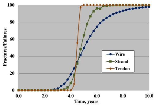
Figure 75. Graph. Plot of the percentage of wire and strand fractures and tendon failures as a function of time based on a mean wire corrosion rate of 15.0 mpy and standard deviation 0.3 of the mean.
