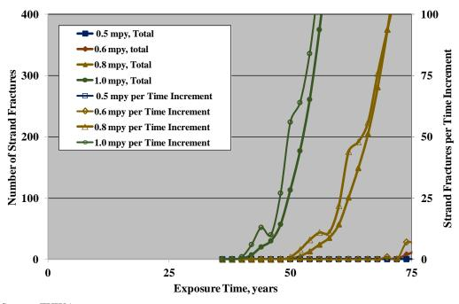
Figure 105. Graph. Number of strand fractures and number per time increment versus time for  $\mu(CRE) = 0.5, 0.6, 0.8,$  and 1.0 mpy and  $\sigma(CRE)/\mu(CRE) = 0.5.$
