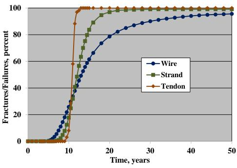
Figure 57. Graph. Plot of the percentage of wire and strand fractures and tendon failures as a function of time based on phase 1 corrosion data for Specimen Number 2.0%–V–S (grout with 2.0 wt% chloride and an air void).<sup>(1)</sup>
