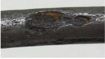
Figure 20. Photo. Example of a more advanced attack on a wire from a single-strand specimen with a grout void from the phase 1 study (figure 243) for which grout chloride concentration was 2.00 wt% (pit depth is 18 mils).<sup>(1)</sup>
