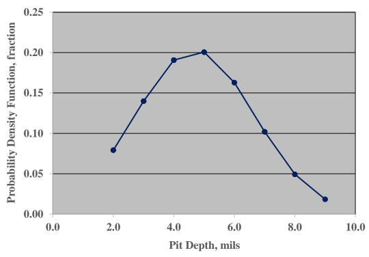
Figure 50. Graph. Normal PDF plot of pit data for depths less than or equal to 9.0 mils for Specimen Number 2.0%–V–S.
