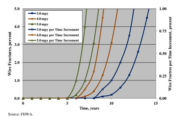
Figure 102. Graph. Percent of wire fractures and percent per time increment versus time for  $\mu(CRE) = 3.0$ , 4.0, and 5.0 mpy and  $\sigma(CRE)/\mu(CRE) = 0.5$ .
