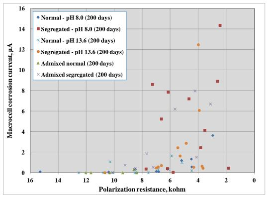
Figure 37. Graph. Rp versus Imacro at 200 d plot.
