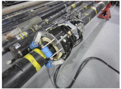
Figure 138. Photo. Permanent magnet-type MMFM device.
