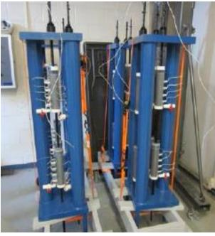
Figure 7. Photo. Grouted single-strand specimens in loading frames.  $^{(1)}$
