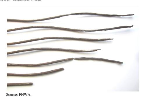
Figure 143. Photo. Cleaned strand sample exhibiting the worst corrosion damage.
