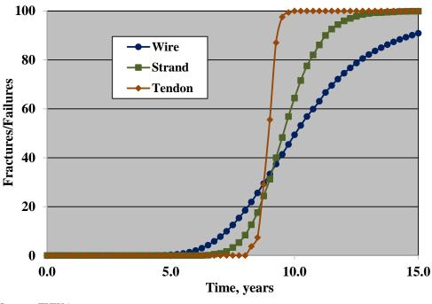
Figure 73. Graph. Plot of the percentage of wire and strand fractures and tendon failures as a function of time based on a mean wire corrosion rate of 7.5 mpy and standard deviation 0.3 of the mean.
