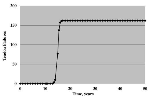
Figure 54. Graph. Plot of the number of tendon failures as a function of time for Specimen Number 1.0%-V-S (grout with 1.0 wt% chloride and an air void).
