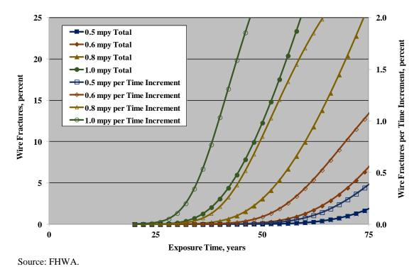
Figure 100. Graph. Percent of wire fractures and percent per time increment versus time for  $\mu(CRE) = 0.5, 0.6, 0.8$ , and 1.0 mpy and  $\sigma(CRE)/\mu(CRE) = 0.5$ .
