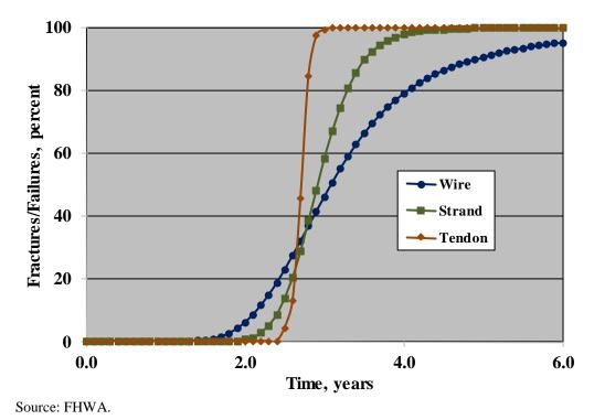
Figure 61. Graph. Plot of the percentage of wire and strand fractures and tendon failures as a function of time based on phase 1 multistrand Specimen Number MS-1.0 (mean corrosion rate 24.8 mpy and standard deviation 8.9).<sup>(1)</sup>
