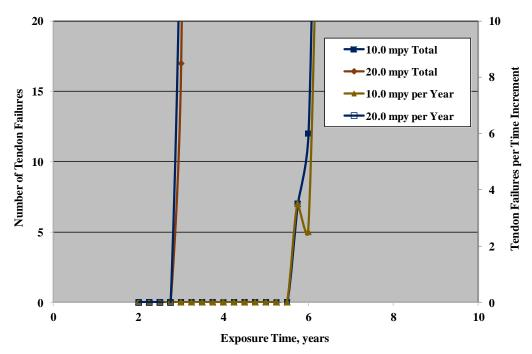
Figure 115. Graph. Number of tendon failures and failures per time increment versus time for  $\mu(CRE)=10.0$  and 20.0 mpy and  $\sigma(CRE)/\mu(CRE)=0.5$ .
