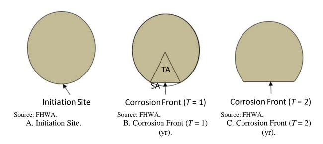
Figure 22. Illustration. Schematic representation of the algorithm employed to project remaining wire cross-section area up to 50-percent loss.
