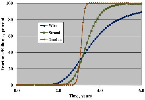
Figure 60. Graph. Plot of the percentage of wire and strand fractures and tendon failures as a function of time based on phase 1 multistrand pit depth distribution data for Specimen Number MS-0.8 (0.80 wt% admixed chloride). (1)
