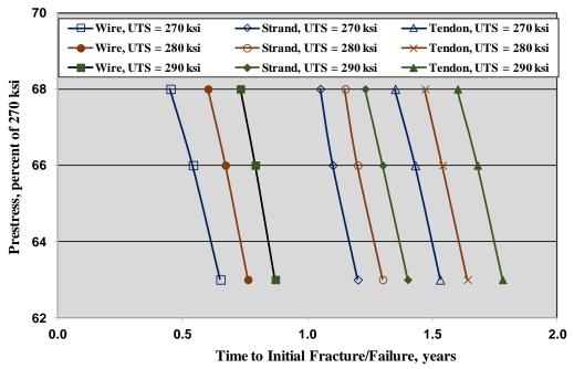
Figure 94. Graph. Plot of  $T_f$  for wires, strands, and tendons as a function of post-tension stress and wire/strand strength for mean corrosion rates of 40.0 mpy and standard deviation 30 percent of the mean.
