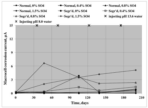
Figure 33. Graph. Mean  $I_{\text{macro}}$  versus time plot for group 2 specimens.
