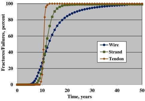
Figure 56. Graph. Plot of the percentage of wire and strand fractures and tendon failures as a function of time based on phase 1 corrosion data for Specimen Number 1.0%–V–US (grout with 1.0 wt% chloride and an air void). (1)
