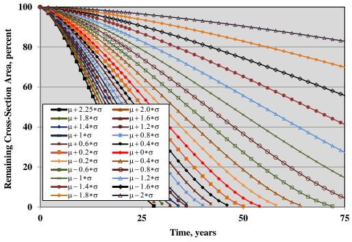
Figure 26. Graph. Projected remaining wire cross-section area as a function of time for a range of  $\mu \pm x \cdot \sigma$  increments.
