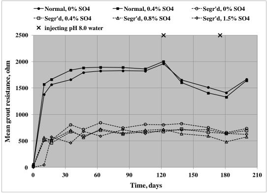
Figure 31. Graph. Mean R versus time plot for group 3 specimens.
