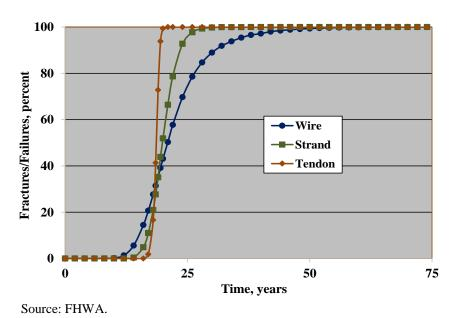
Figure 43. Graph. Plot of the percentage of wire and strand fractures and tendon failures as a function of time for the case of sound grout with 0.80 wt% chloride and  $\sigma(CRE)$  on corrosion rate equal to 0.30  $\mu(CRE)$ .
