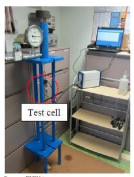
Figure 3. Photo. Load frame and cell for loading single-wire specimens. (1)
