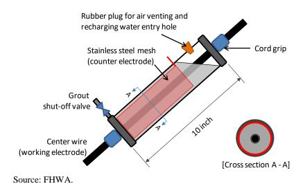
Figure 10. Illustration. Schematic of test specimen containing an artificial void.
