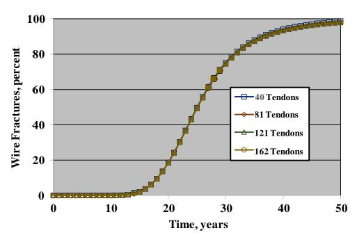
Figure 95. Graph. Plot of the percentage of wire fractures as a function of time for systems with 40, 81, 121, and 162 tendons.
