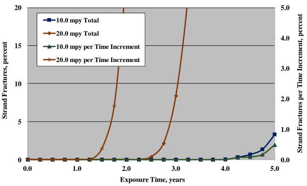
Figure 110. Graph. Percent of strand fractures and percent per time increment versus time for  $\mu(CRE)$  =10.0 and 20.0 mpy and  $\sigma(CRE)/\mu(CRE)$  = 0.5.
