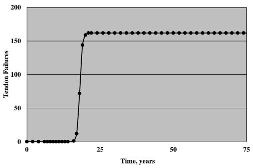
Figure 40. Graph. Number of tendon failures as a function of time for the case of sound grout with 0.80 wt% chloride based on pit depth determinations for phase 1 Specimen Number 0.8%–F–S. $^{(1)}$
