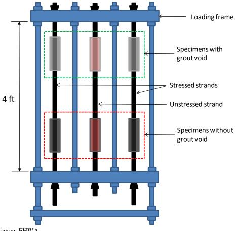
Figure 6. Illustration. Schematic representation of grouted single-strand specimens in a loading frame.  $^{(1)}$
