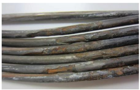
Figure 16. Photo. Corroded wires of a strand as reproduced from figure 217 from the phase  $1 \text{ study.}^{(1)}$
