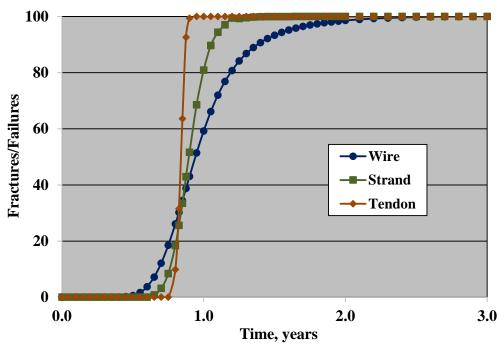
Figure 81. Graph. Plot of the percentage of wire and strand fractures and tendon failures as a function of time based on a mean wire corrosion rate of 80.0 mpy and standard deviation 0.3 of the mean.
