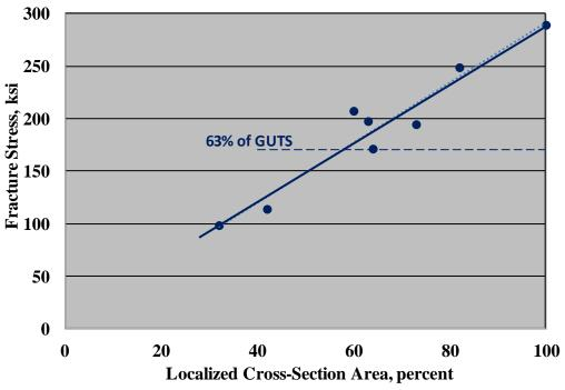
Figure 15. Graph. Plot of prestressing steel wire fracture stress (FS) as a function of the remaining cross-section area (RCSA) of the wire at the most corroded location.
