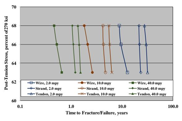
Figure 91. Graph. Plot of  $T_f$  for wires, strands, and tendons as a function of post-tension stress for mean corrosion rates of 2.0, 10.0, and 40.0 mpy and standard deviation 0.3 of the mean.
