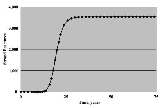
Figure 39. Graph. Number of strand fractures as a function of time for the case of sound grout with 0.80 wt% chloride based on pit depth determinations for phase 1 Specimen Number 0.8%–F–S.<sup>(1)</sup>
