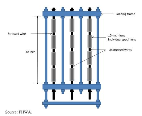
Figure 14. Illustration. Specimen arrangement for the ambient exposure testing.
