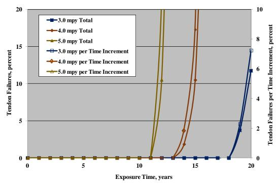
Figure 114. Graph. Percent of tendon failures and percent per time increment versus time for  $\mu(CRE) = 3.0$ , 4.0, and 5.0 mpy and  $\sigma(CRE)/\mu(CRE) = 0.5$ .
