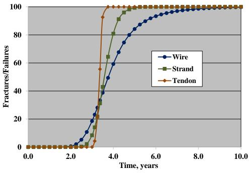
Figure 76. Graph. Plot of the percentage of wire and strand fractures and tendon failures as a function of time based on a mean wire corrosion rate of 20.0 mpy and standard deviation 0.3 of the mean.
