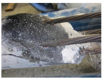
Figure 59. Photo. Appearance of black deposits at the void/grout interface as shown by figure 213 from the phase 1 report.<sup>(1)</sup>
