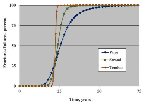
Figure 70. Graph. Plot of the percentage of wire and strand fractures and tendon failures as a function of time based on a mean wire corrosion rate of 3.0 mpy and standard deviation 0.3 of the mean.
