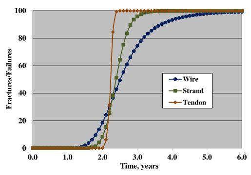
Figure 77. Graph. Plot of the percentage of wire and strand fractures and tendon failures as a function of time based on a mean wire corrosion rate of 30.0 mpy and standard deviation 0.3 of the mean.
