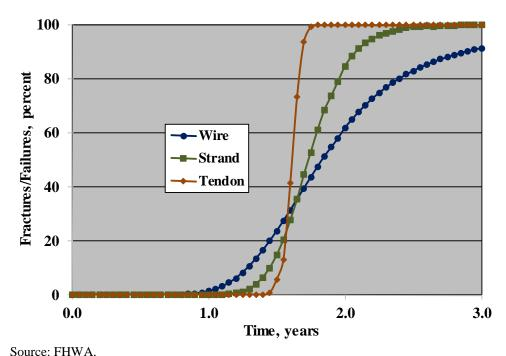
Figure 64. Graph. Plot of the percentage of wire and strand fractures and tendon failures as a function of time based on phase 1 multistrand Specimen Number MS-2.0 (2.00 wt% admixed chloride). (1)
