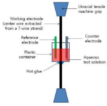
Figure 2. Illustration. Schematic representation of the testing arrangement for single-wire specimens. $^{(1)}$
