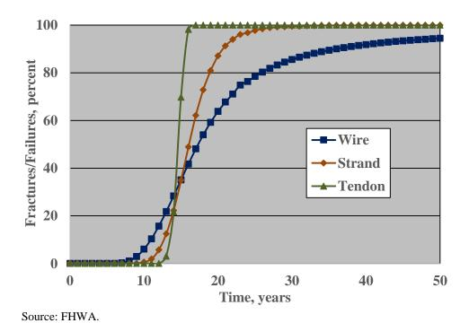
Figure 135. Graph. Plot of projected wire and strand fractures and tendon failures as a function of time for a mean chloride concentration of 2.50 wt% cement and standard deviation 2.24.
