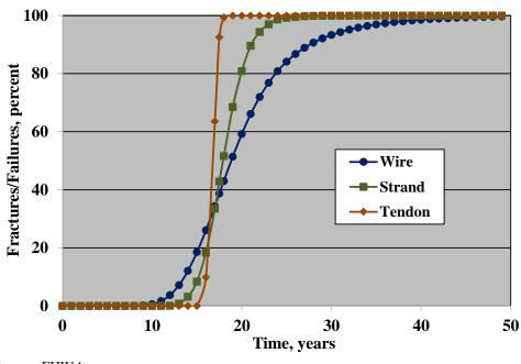
Figure 71. Graph. Plot of the percentage of wire and strand fractures and tendon failures as a function of time based on a mean wire corrosion rate of 4.0 mpy and standard deviation 0.3 of the mean.
