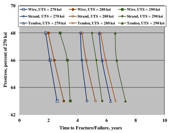
Figure 93. Graph. Plot of  $T_f$  for wires, strands, and tendons as a function of post-tension stress and wire/strand strength for mean corrosion rates of 10.0 mpy and standard deviation 0.3 of the mean.
