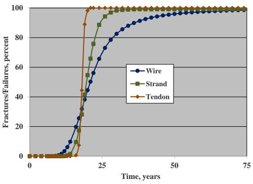
Figure 41. Graph. Combined plot of the percentage of wire and strand fractures and tendon failures as a function of time based on pit depth determinations for phase 1 Specimen Number 0.8%–F–S. $^{(1)}$
