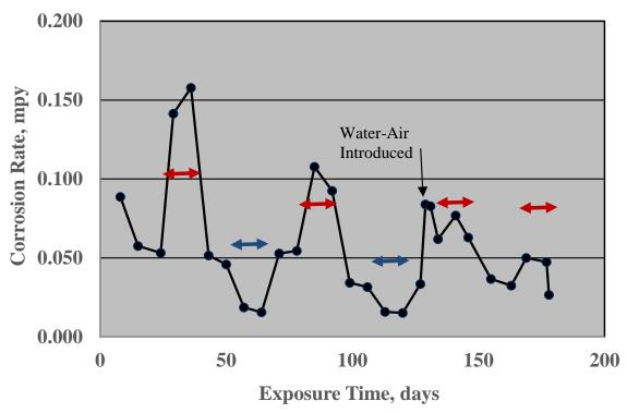
Figure 47. Graph. Plot of corrosion rate versus time for Specimen Number 2.0%-V-S.
