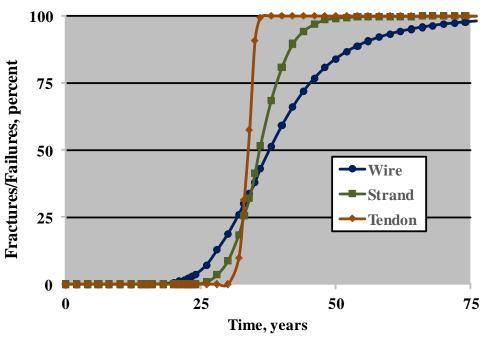
Figure 69. Graph. Plot of the percentage of wire and strand fractures and tendon failures as a function of time based on a mean wire corrosion rate of 2.0 mpy and standard deviation 0.3 of the mean.
