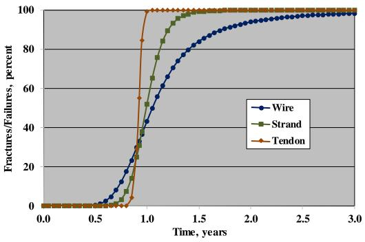
Figure 63. Graph. Plot of the percentage of wire and strand fractures and tendon failures as a function of time based on measurements made on phase 1 multistrand Specimen Number  $MS-0.4~(0.4~wt\%~admixed~chloride).^{(1)}$
