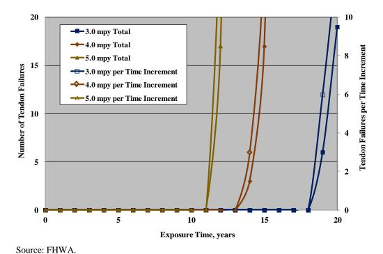
Figure 113. Graph. Number of tendon failures and failures per time increment versus time for  $\mu(CRE) = 3.0, 4.0,$  and 5.0 mpy and  $\sigma(CRE)/\mu(CRE) = 0.5.$
