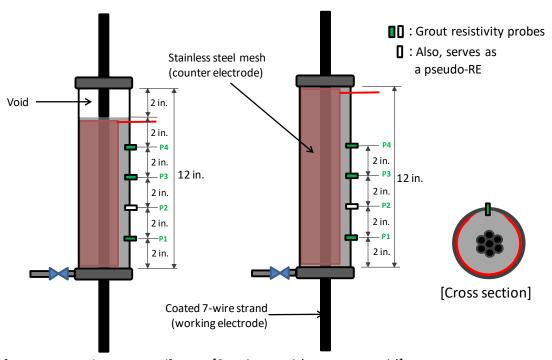
[Specimen with grout void]
