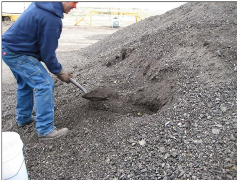
Figure 19. Photo. Sampling RAP from the stockpile.
