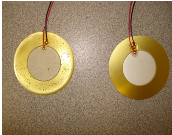
Figure 111. Photo. Piezoelectric transducer covered with a layer of rubber.
