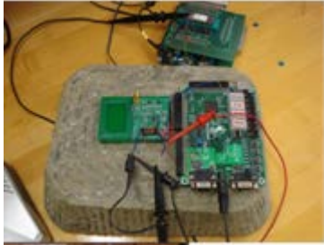
Figure 69. Photo. Receiver placed on top of the concrete specimen.
