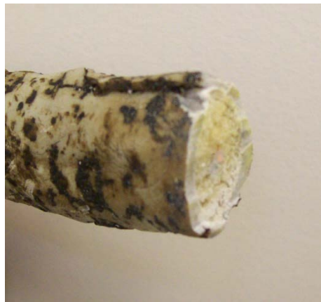
Figure 133. Photo. Material specimen recovered from the asphalt beam after compaction.
