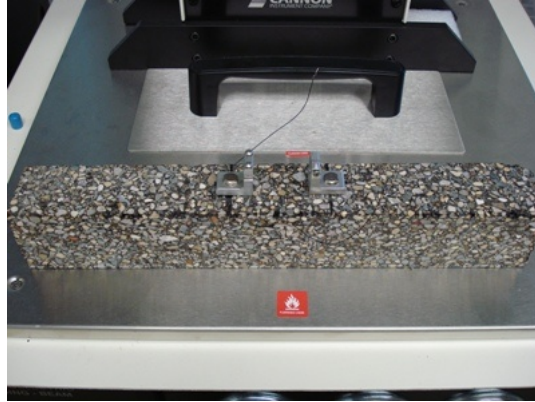
Figure 108. Photo. Cut asphalt specimen with embedded piezoelectric generator.
