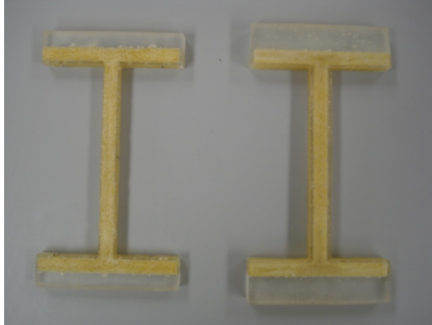
Figure 142. Photo. Tested prototypes of piezoelectric transducer embedded in epoxy and coated with a polyurethane thermal insulator.
