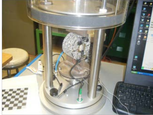
Figure 83. Photo. Experimental setup for the indirect tensile test.
