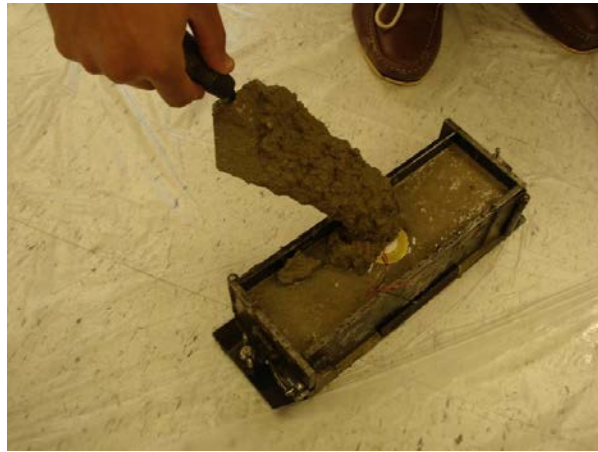
Figure 110. Photo. Piezoelectric transducer embedded in concrete.
