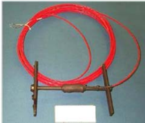
Figure 118. Photo. Example of commercially available asphalt strain gauge.
