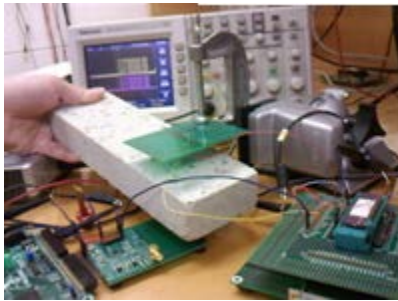
Figure 70. Photo. Concrete specimen placed between a reader and receiver.
