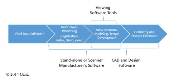
Figure 7. Flowchart. Point cloud processing pipeline (after Gant). (9)
