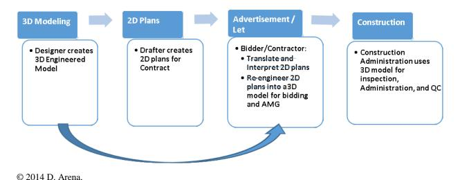
Figure 14. Flowchart. Traditional 2D design workflow versus 3D workflow (after Arena). (41)
