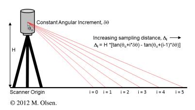
Figure 5. Diagram. A terrestrial static LiDAR system. (7)
