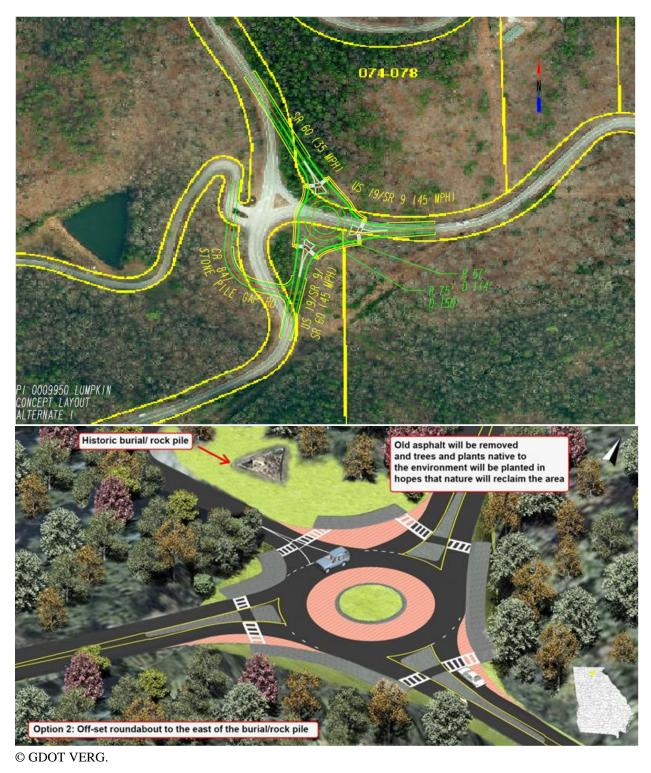
Figure 22. Diagrams. Comparison between 2D plan view and visualization with 3D modeling for Option 2: Offset Roundabout.
