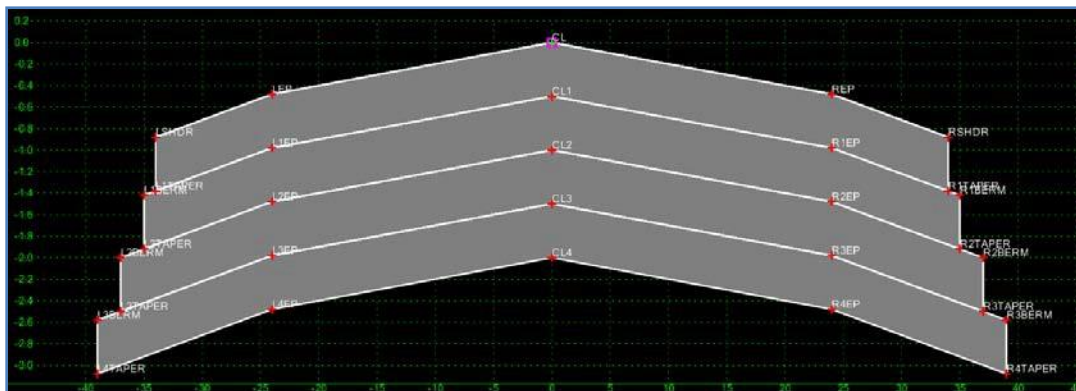
Figure 18. Illustration. CADD template representing a two-lane road with shoulders.
