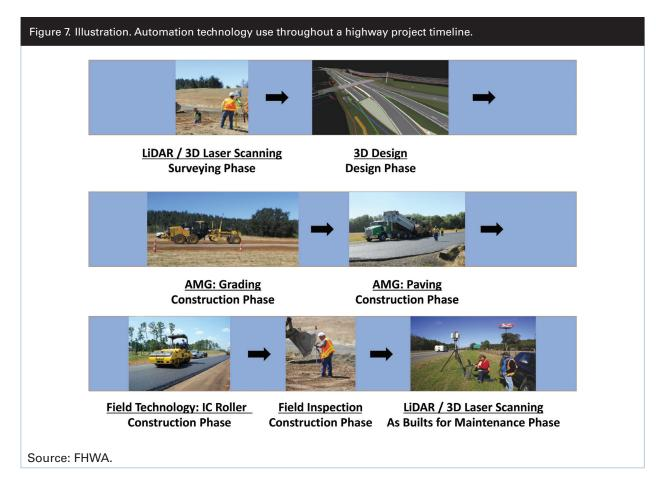
applications. It also depends on accurate survey control, which allows 3D data to be associated with a geographic coordinate system and consolidated.
