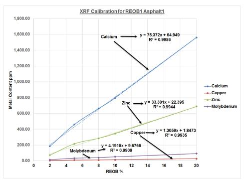
Figure 3. Typical Calibration Curves for REOB Asphalt Blends.
