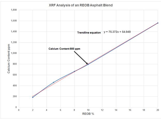
Figure 1. Calcium Analysis of Asphalt Blends Containing REOB.
