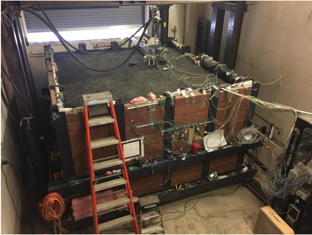
Figure 84. Photo. Completed large-scale-box test setup for experiment No. 5—loading location A (top of steel pipe).
