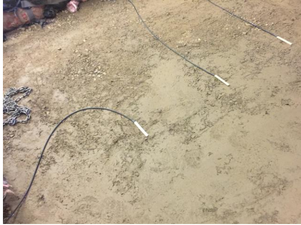
Figure 62. Photo. Asphalt strain gauges placed on top of the CAB.
