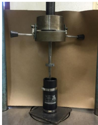
Figure 21. Photo. Static compaction of triaxial test specimen.
