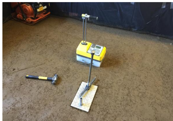
Figure 28. Photo. Nuclear density gauge instruments on top of a compacted lift of SG soil.
