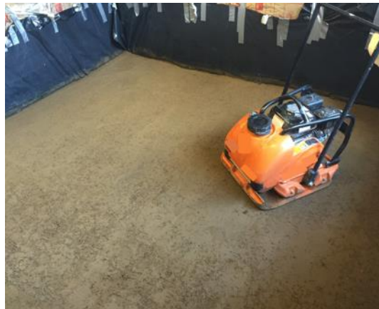
Figure 27. Photo. Compaction of SG soil to target density using a vibratory-plate compactor.
