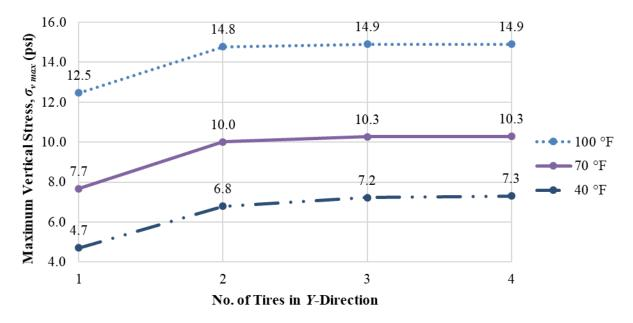
Figure 72. Chart.  $\sigma_{v max}$  change with tires in y-direction for three temperatures.
