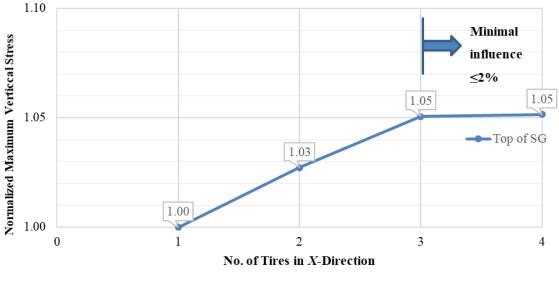
Figure 58. Chart. Change in normalized  $\sigma_{v max}$  with added tires in x-direction (SHL case No. 1: LA-4T-1, 100 °F, PS 1).
