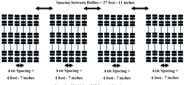
Length of Vehicle = 205 foot - 4.8 inches Width of Vehicle = 17 foot - 5.8 inches
