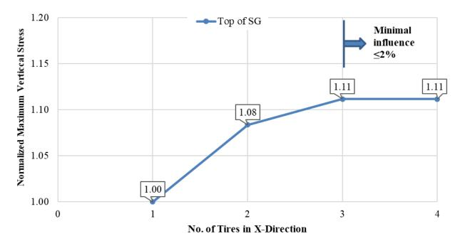
Figure 34. Chart. Normalized  $\sigma_{v max}$  as a function of number of tires in *x*-direction (SHL case No. 2: LA-8T-14, 100 °F, PS 2).
