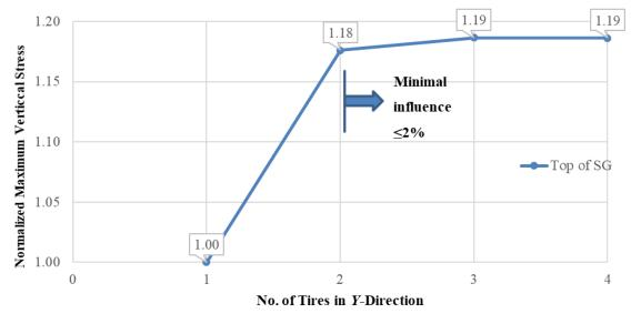
Figure 60. Chart. Change in normalized  $\sigma_{v max}$  with added tires in y-direction (SHL case No. 1: LA-4T-1, 100 °F, PS 1).
