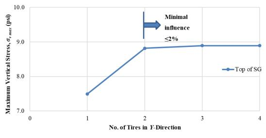
Figure 59. Chart. Change in  $\sigma_{v max}$  with added tires in y-direction (SHL case No. 1: LA-4T-1, 100 °F, PS 1).
