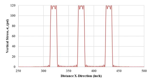
Figure 25. Chart.  $\sigma_v$  distribution on top of AC (z = 0 inch), three tires (SHL case No. 2: LA-8T-14, 100 °F, PS 2).
