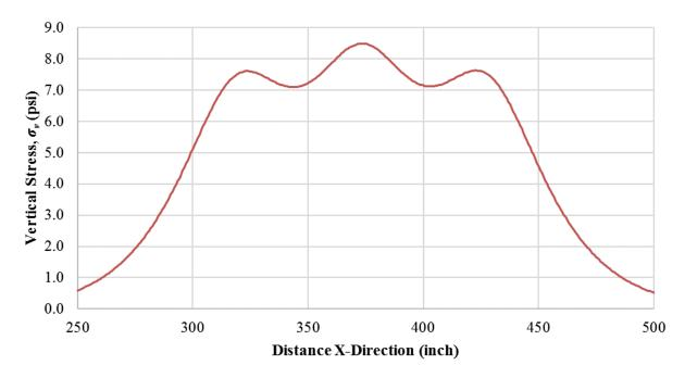
Figure 28. Chart.  $\sigma_v$  distribution at 12 inches below SG (z = 31 inches), three tires (SHL case No. 2: LA-8T-14, 100 °F, PS 2).
