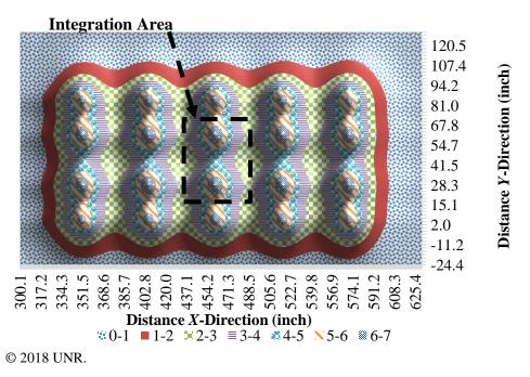
Figure 68. Chart. σ<sub>ν</sub> distribution on top of SG four by four tires (SHL case No. 3: LA-12T-16, 100 °F, PS 1)—top view.
