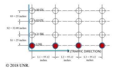
Figure 22. Illustration. Incremental tire-load approach—four tires (red-filled circles).
