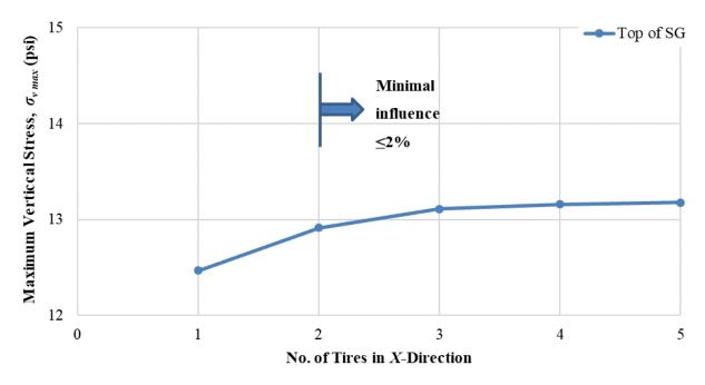
Figure 42. Chart. Change in  $\sigma_{v max}$  with added tires in *x*-direction (SHL case No. 2: LA-8T-14, 100 °F, PS 1).
