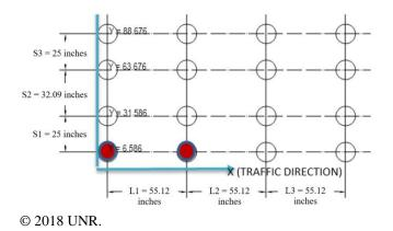
Figure 20. Illustration. Incremental tire-load approach—two tires (red-filled circles).
