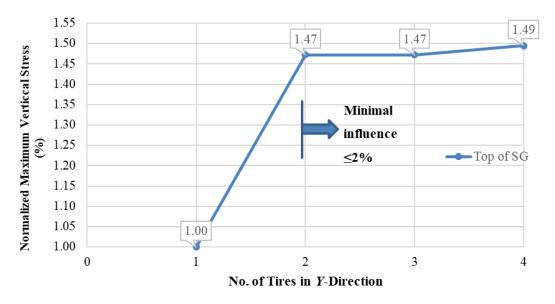
Figure 53. Chart. Change in normalized  $\sigma_{v max}$  with added tires in y-direction (SHL case No. 2: LA-8T-14, 100 °F, PS 3).
