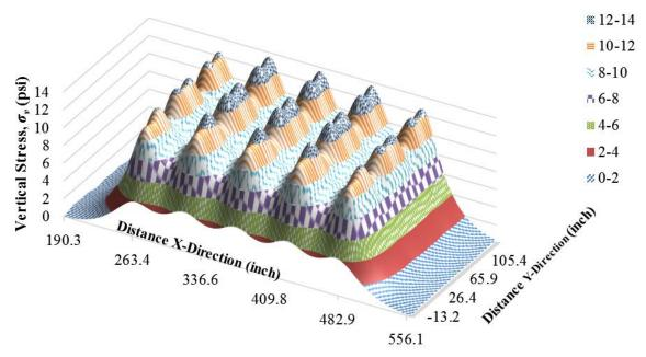
Figure 37. Chart.  $\sigma_{\nu}$  distribution on top of SG five by six tires (SHL case No. 2: LA-8T-14, 100 °F, PS 2)—3D view.
