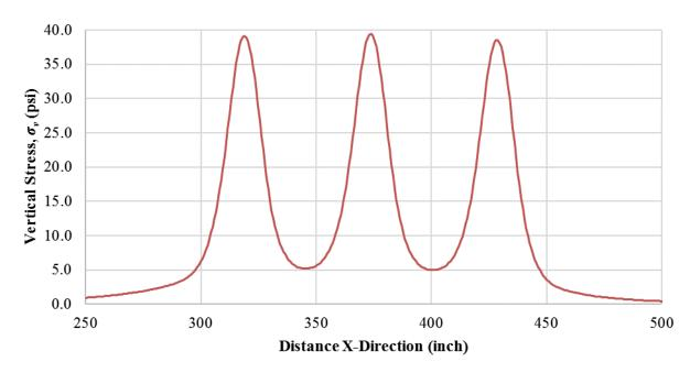
Figure 26. Chart.  $\sigma_{\nu}$  distribution on top of CAB (z = 9 inches), three tires (SHL case No. 2: LA-8T-14, 100 °F, PS 2).
