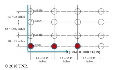
Figure 21. Illustration. Incremental tire-load approach—three tires (red-filled circles).
