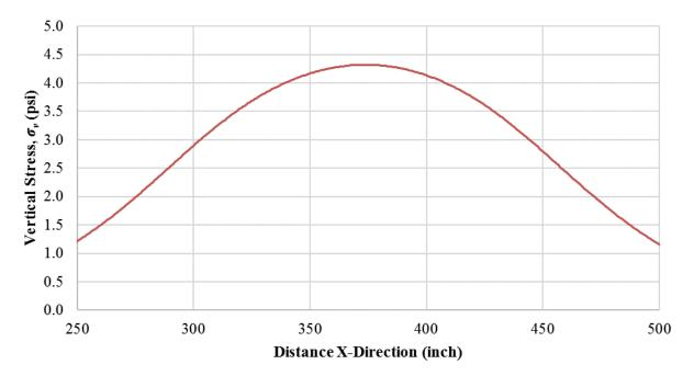
Figure 29. Chart.  $\sigma_v$  distribution at 72 inches below SG (z = 91 inches), three tires (SHL case No. 2: LA-8T-14, 100 °F, PS 2).
