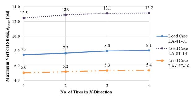
Figure 69. Chart. Change in  $\sigma_{v max}$  with added tires in *x*-direction (all SHL cases, 100 °F, PS 1).
