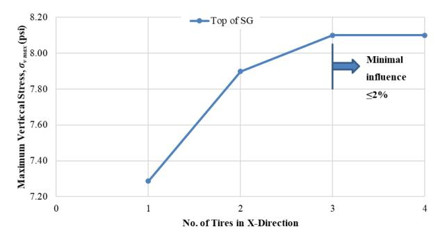
Figure 33. Chart. Change in  $\sigma_{v max}$  with multiple tires in *x*-direction (SHL case No. 2: LA-8T-14, 100 °F, PS 2).
