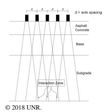
Figure 15. Illustration. Five-line model for SHL simulation—elevation view.
