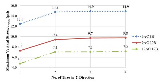
Figure 56. Chart. Change in  $\sigma_{y max}$  with added tires in y-direction (SHL case No. 2: LA-8T-14, 100 °F, all PSs).
