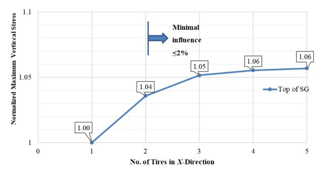
Figure 43. Chart. Change in normalized  $\sigma_{v max}$  with added tires in x-direction (SHL case No. 2: LA-8T-14, 100 °F, PS 1).
