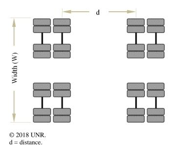
Figure 3. Illustration. Double-dolly configuration according to CDOT.
