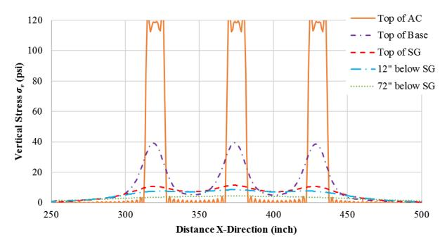
Figure 30. Chart.  $\sigma_{\nu}$  distribution at various depths below pavement surface, three tires (SHL case No. 2: LA-8T-14, 100 °F, PS 2).
