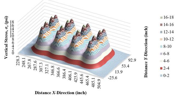
Figure 47. Chart.  $\sigma_{\nu}$  distribution on top of SG four by four tires (SHL case No. 2: LA-8T-14, 100 °F, PS 1)—3D view.
