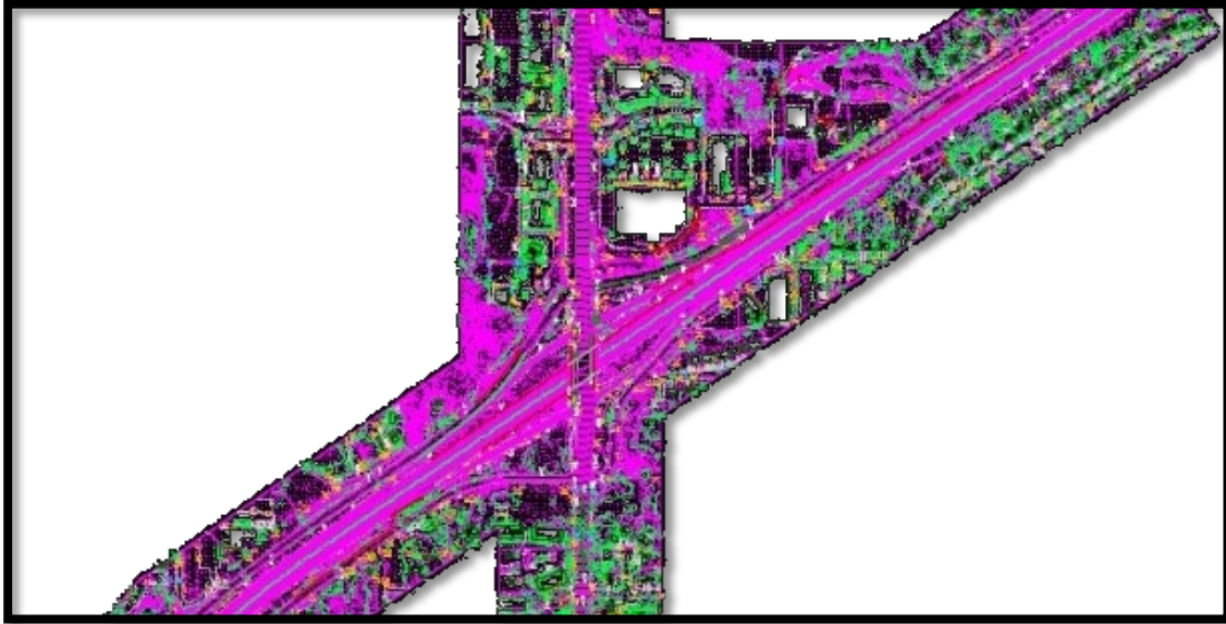
Figure 5. Screen capture. Typical topographic file created from LiDAR data.
