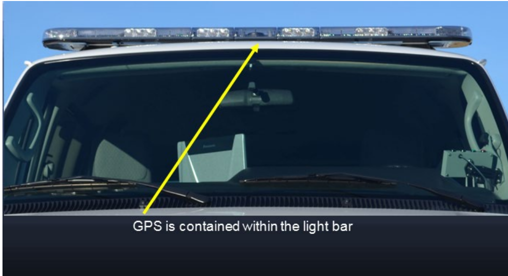
Figure 15. Photo. Location of the GPSR.
