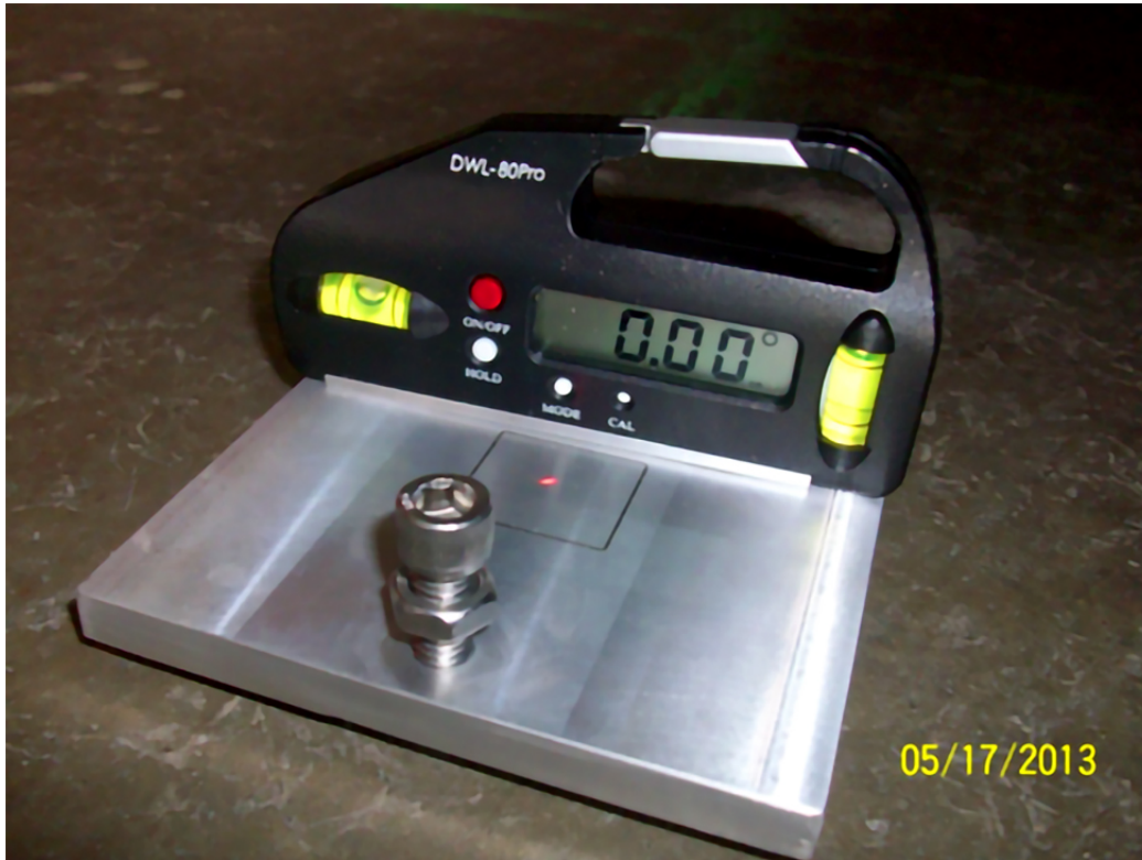
Figure 83. Photo. Digital level.
