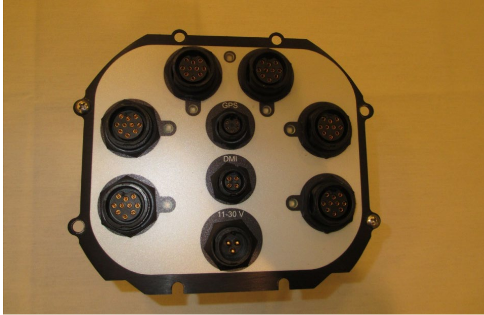
Figure 7. Photo. Ports on the DAU.
