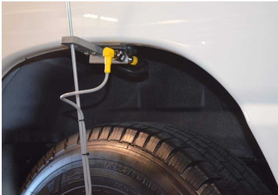
Figure 12. Photo. DMI encoder.
