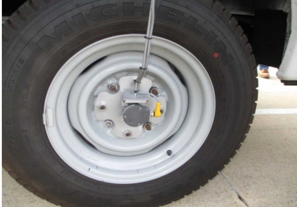
Figure 12. Photo. DMI encoder.
