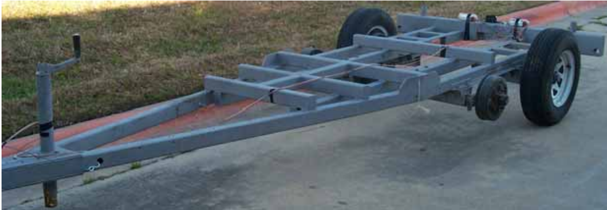
Figure 4. Stripped and sandblasted trailer ready to go to powder coat facility.
