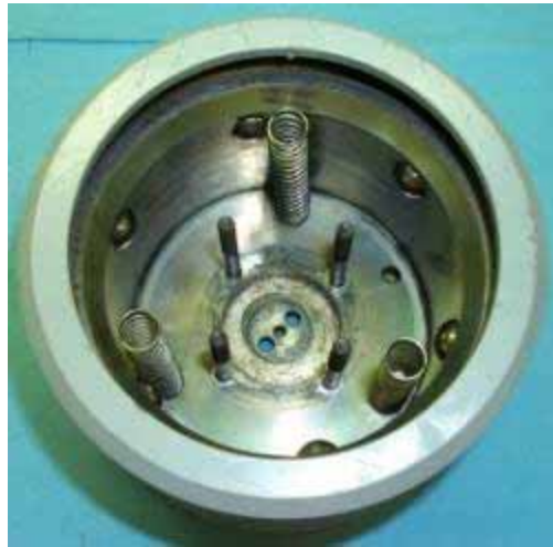
Figure 75. Interior of catch assembly with compression springs.
