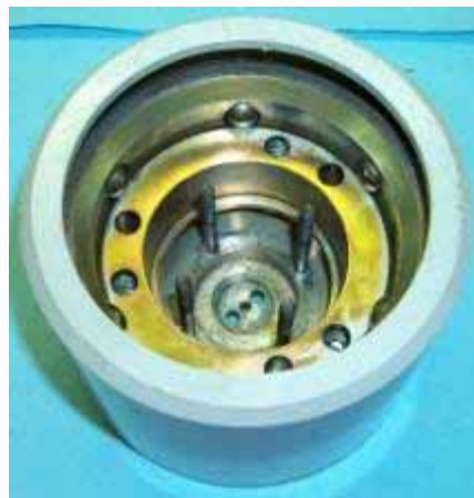
Figure 78. Inner ring in position inside the outer shell.
