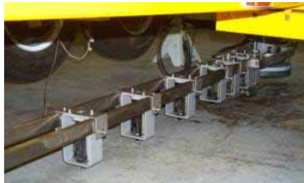
Figure 109. Completed assembly of raise/lower bar.
