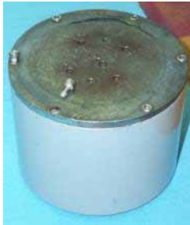
Figure 73. Inner catch top cover installed.
