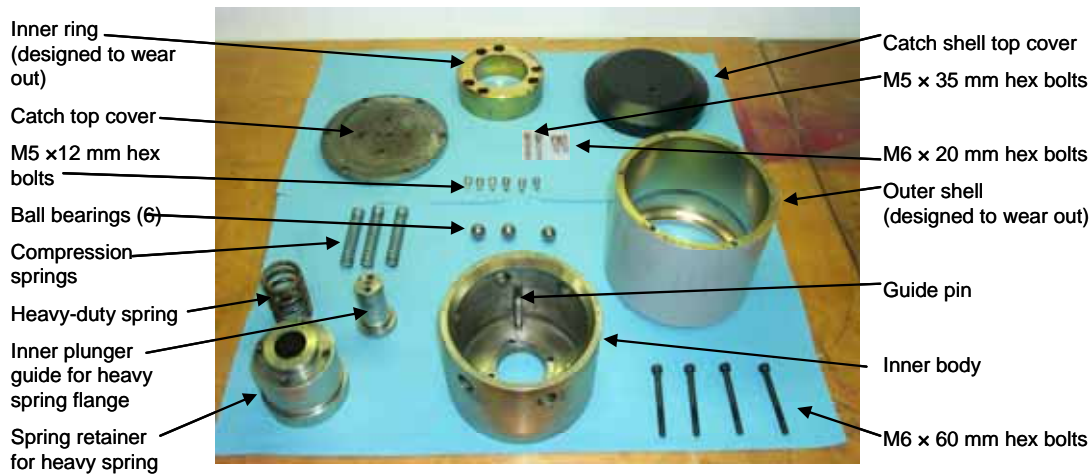
Figure 66. Upper catch shell and interior components.
