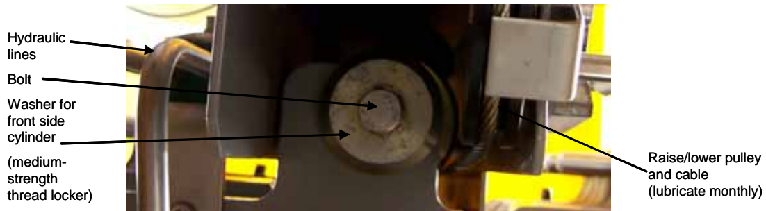
Figure 88. Front side cylinder, looking up, from under FWD.
