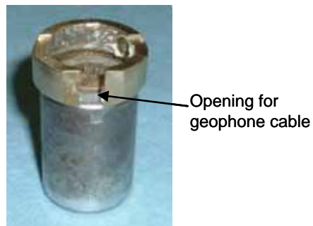
Figure 115. Mounted ground ring.
