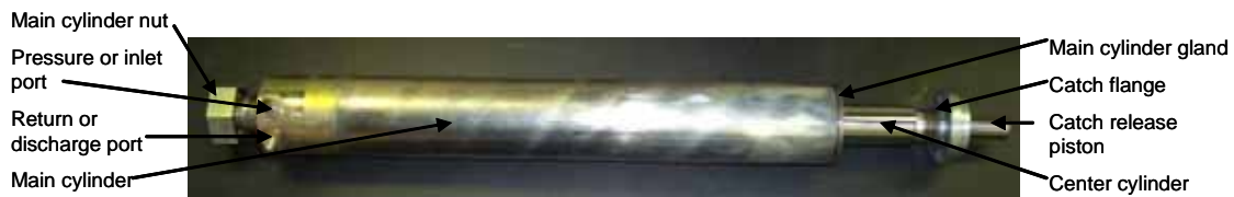
Figure 63. Assembled main cylinder.
