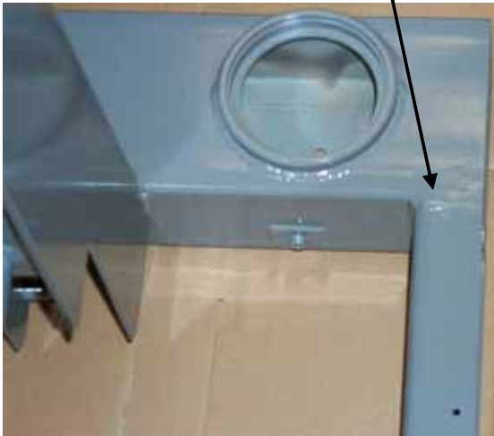
Subassembly top joint reinforced weld
