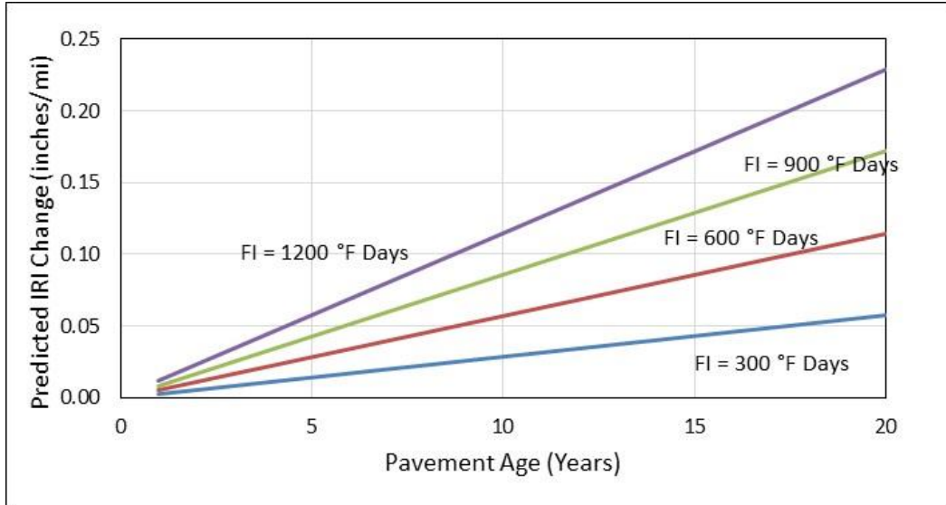
Figure 6. Graph. Increase in IRI due to FI predicted by the MEPDG model for four different average annual FI values.
