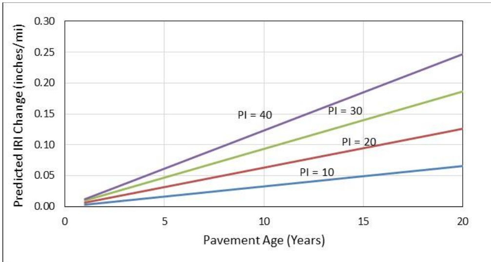
Figure 4. Graph. Increase in IRI due to PI of subgrade predicted by the MEPDG model for four different PI values.
