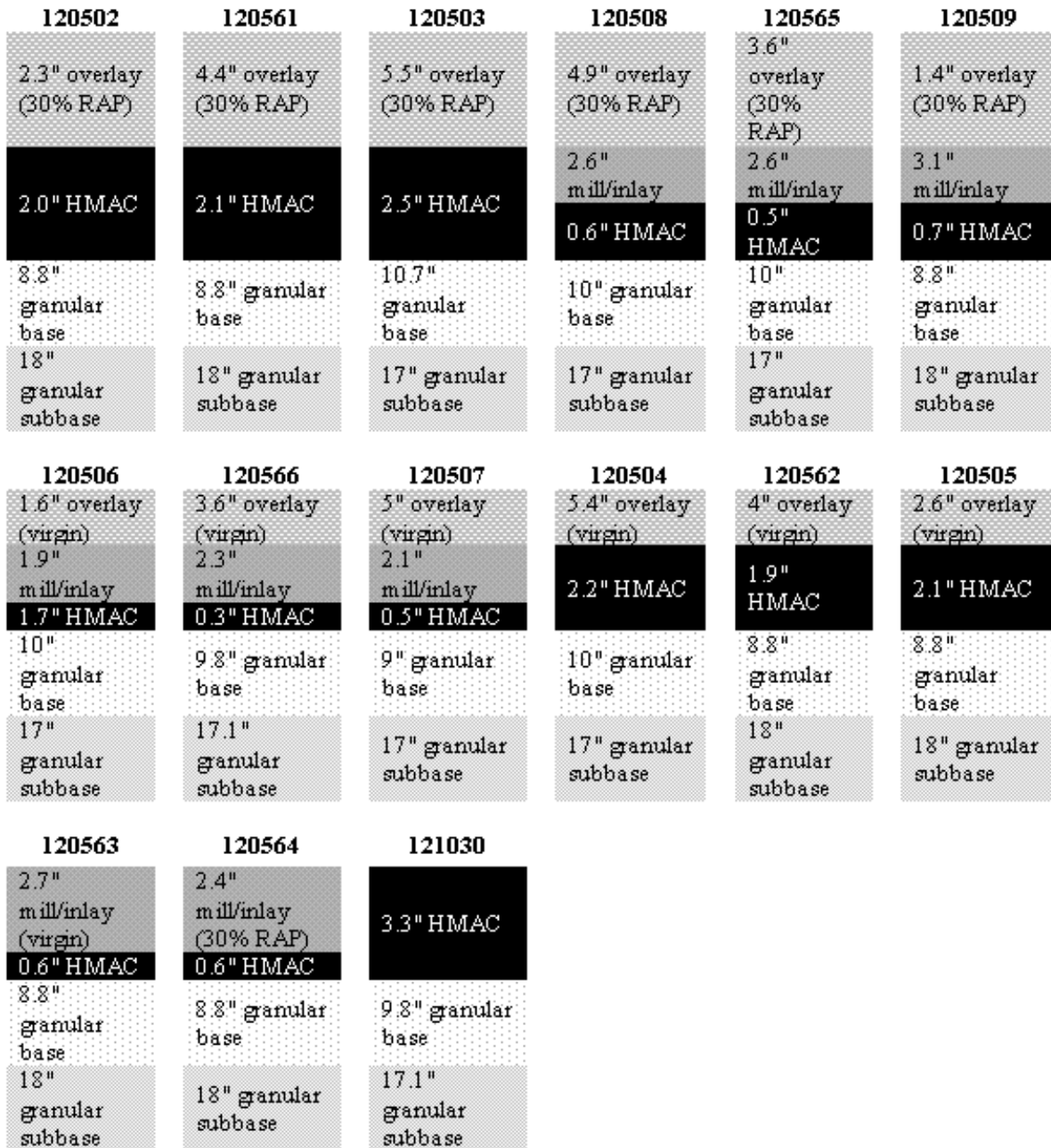
Figure 8. Illustration. Pavement structure in Florida SPS-5 test sections.
